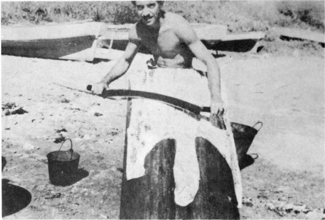
FIG. 7 - FLESHING A SKIN ON THE BEAMING BOARD.
