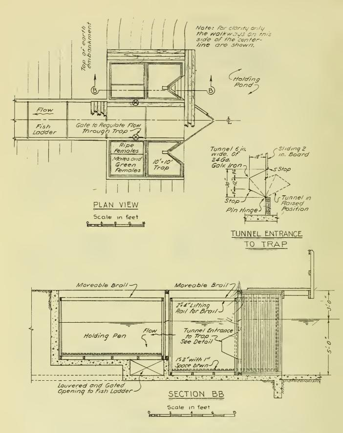
Figure 4:--Design drawings of downstream trapping system including trap and holding pen. Details of the tunnel entrance and flow pattern are shown.
