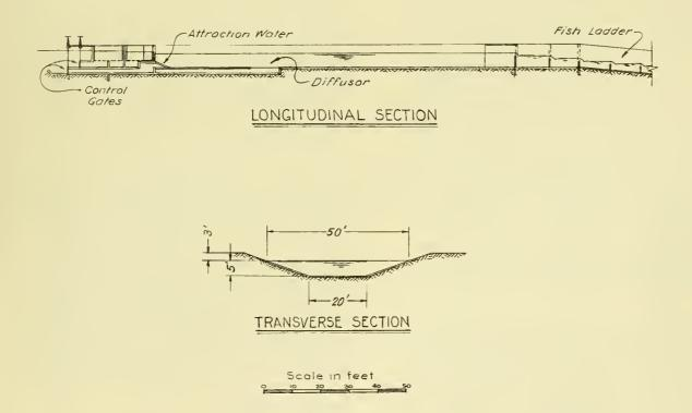
Figure 1:--Design drawings of a single holding pond giving dimensions of the pond, method of water introduction and withdrawal, and location of the trapping facilities.
