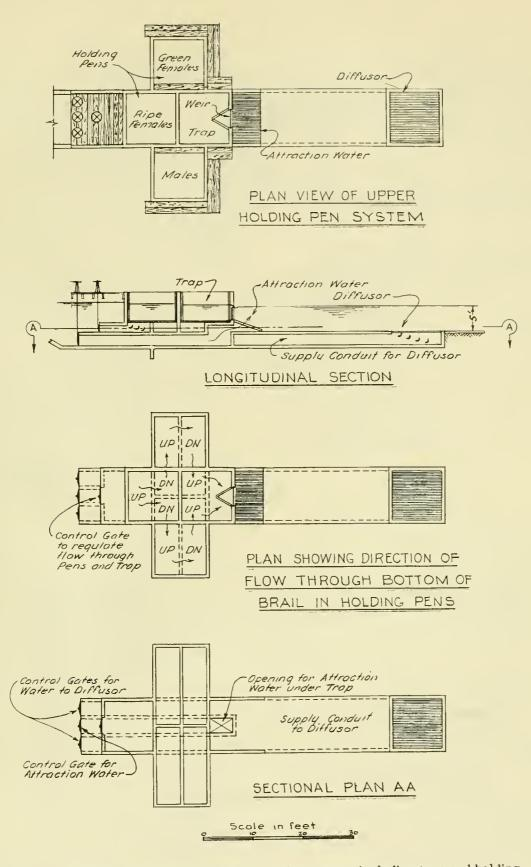
Figure 3:--Design drawings of upstream trapping system including trap and holding pens. The water path through the holding pens and trap is indicated.
