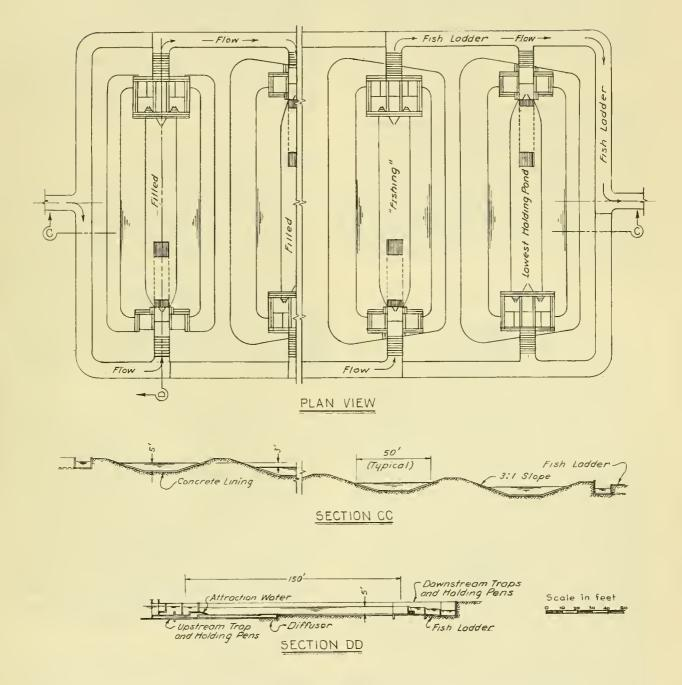
Figure 2:--Plan for operation of holding ponds in series showing double fishway system.
