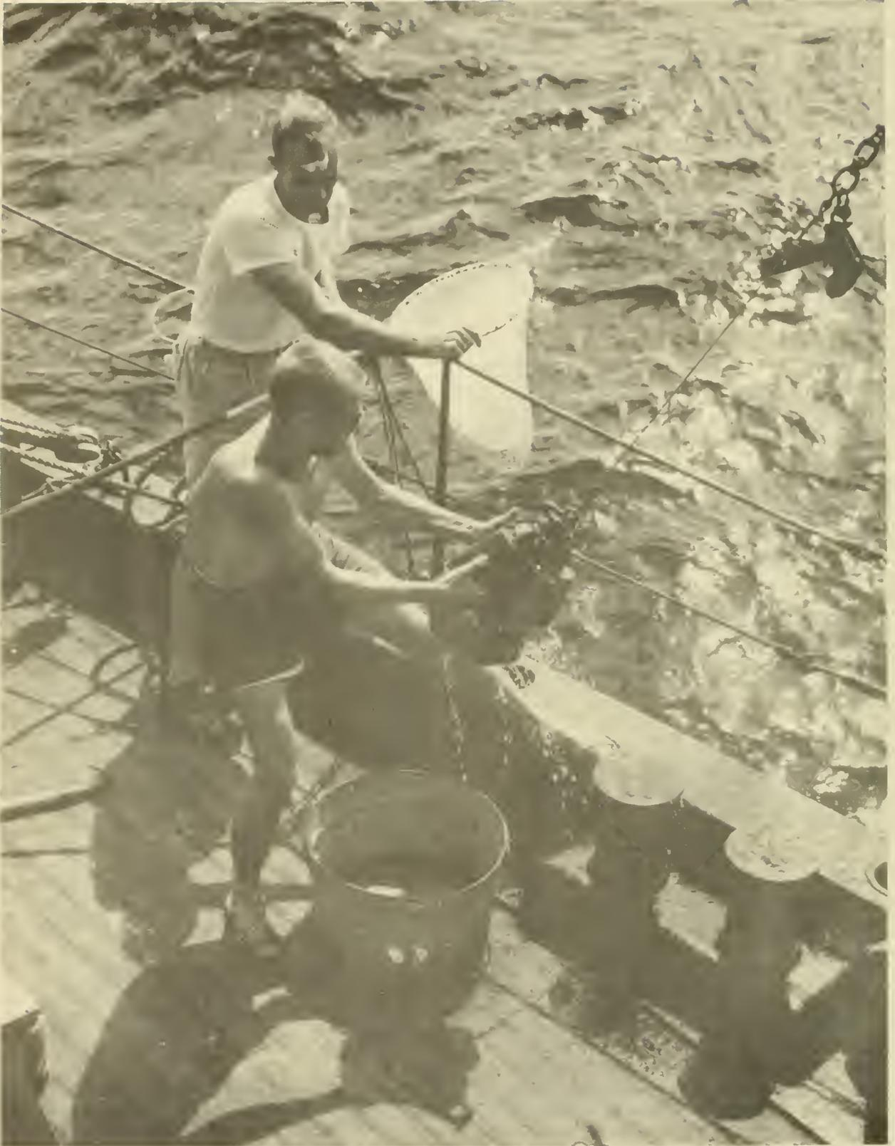
Figure 2.--Modified orange-peel bottom sampler.
