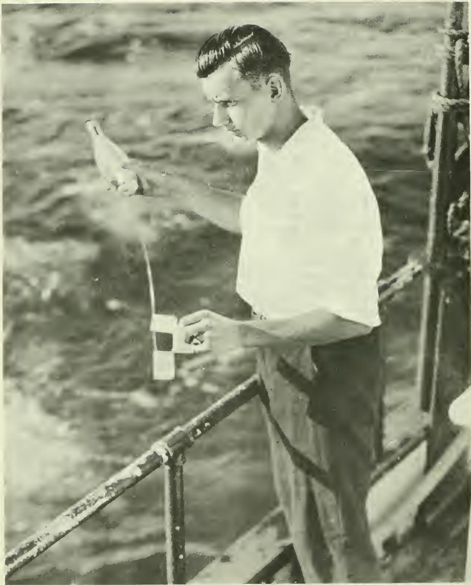
Figure 1.--Drift bottle with a metal drag, was deposited from the research vessel *Fulmar*.
