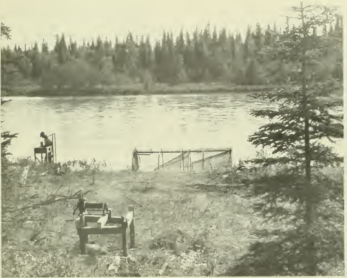
Figure 3.--Hand winch used to roll fyke traps out of river.
