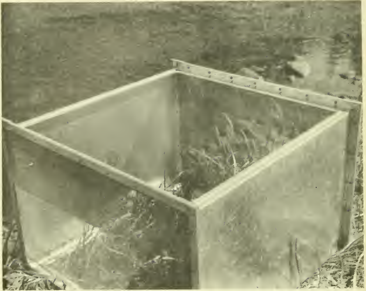
Figure 8.--Quadrat sampler used in intertidal fry studies.
