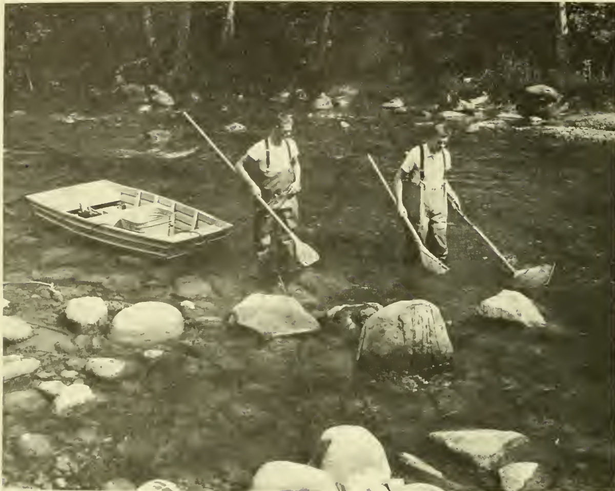
Figure 9.--Fishing with the Type IV shocker by wading. Note use of polaroid glasses by the biologists for locating fish.
