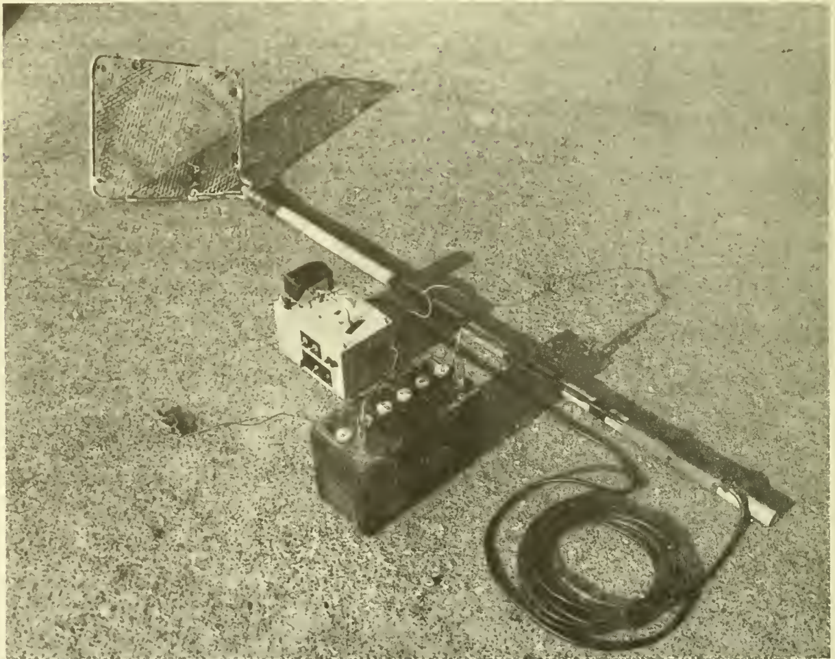
Figure 1.--The Type IV shocker in operational condition, less the cathode. The strip-switch mounting is on the anode handle. The small black box on the shocker is the running-time meter.
