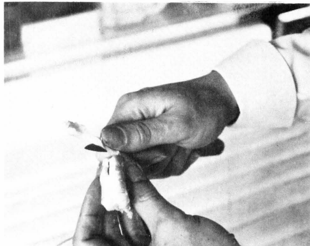
3. Removing sand vein
