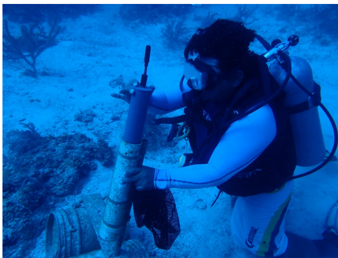
Diver installs a passive acoustic recorder on a coral reef.
