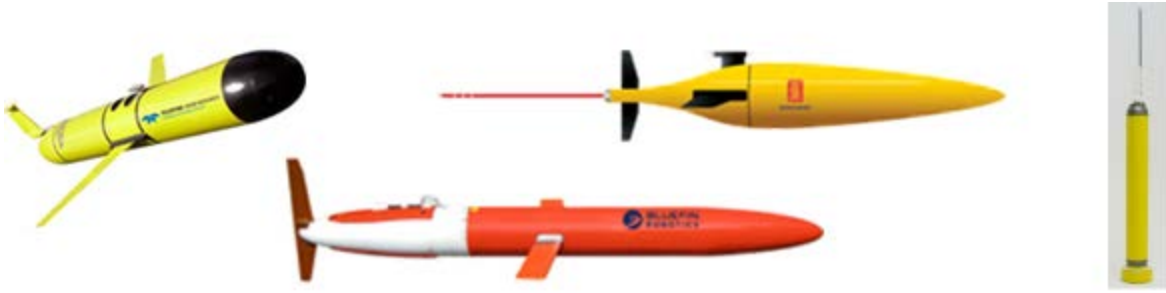
Figure 10. Buoyancy gliders (L-R from Teledyne, Bluefin Robotics, and Kongsberg) and buoyancy floats (e.g., right, https://argo.ucsd.edu/ ) collect oceanographic data over months to years and telemeter the data and their positions to researchers ashore via satellite.
