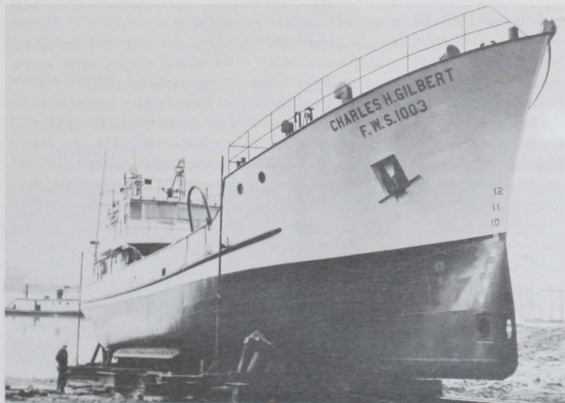
Figure 20. --Underwater observation chamber in bow of Charles H. Gilbert .
