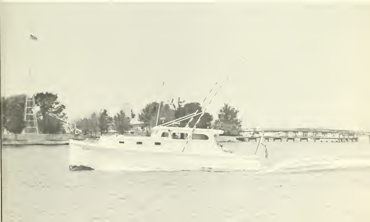
The cabin cruiser carries a laboratory, depth recorder, and two-way radio
