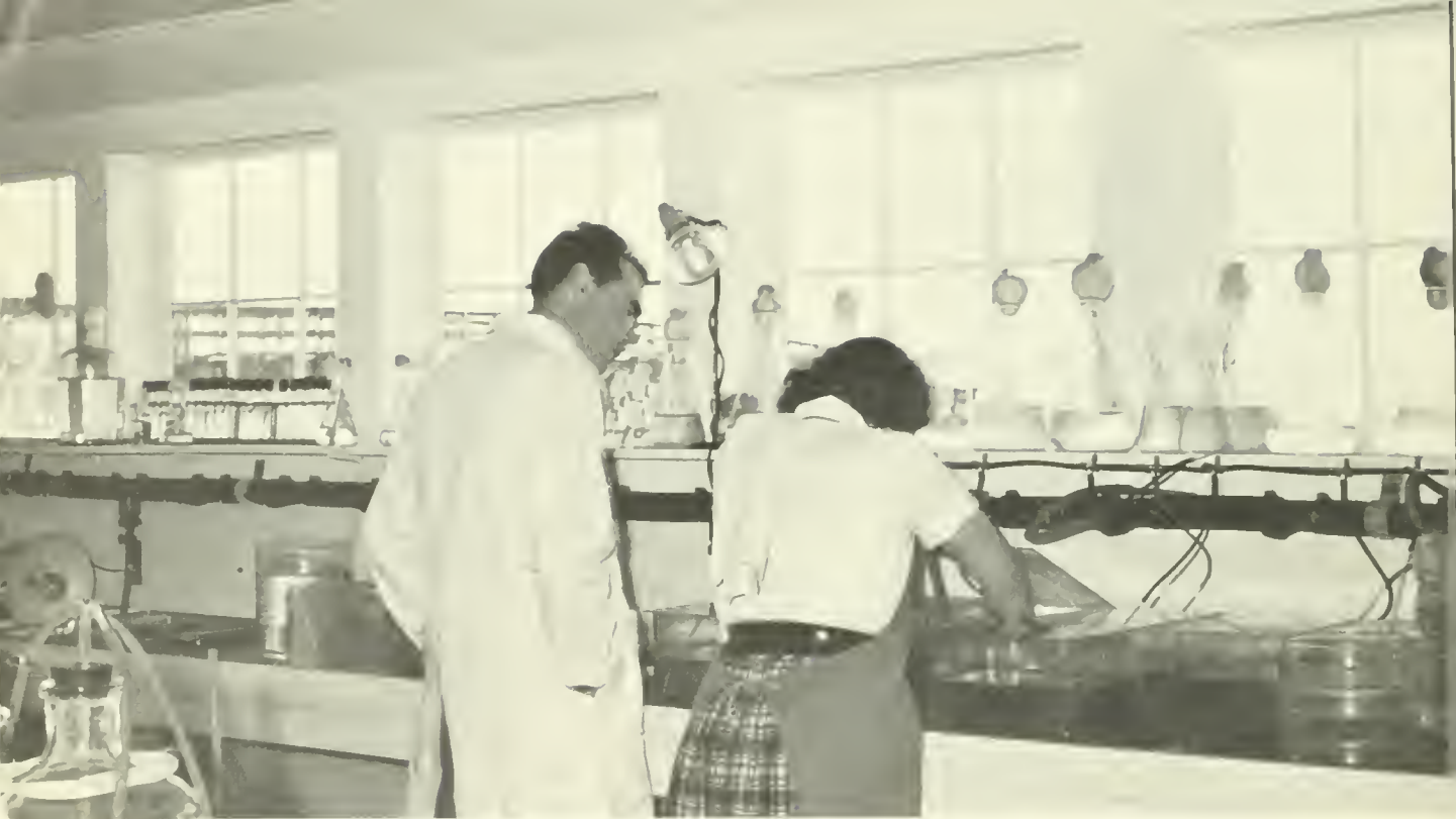
A plastic pipe brings sea water direct to the salt-water culture room. Here, fish and the larger invertebrates, such as shrimp and crabs, are raised and held
