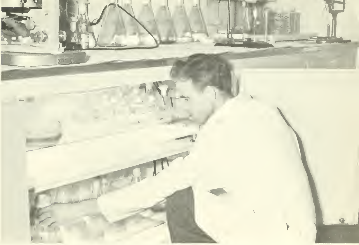
Constant light and temperature cabinet in the plankton-culture laboratory, where bacteria, marine algae, and other marine organisms are cultured
