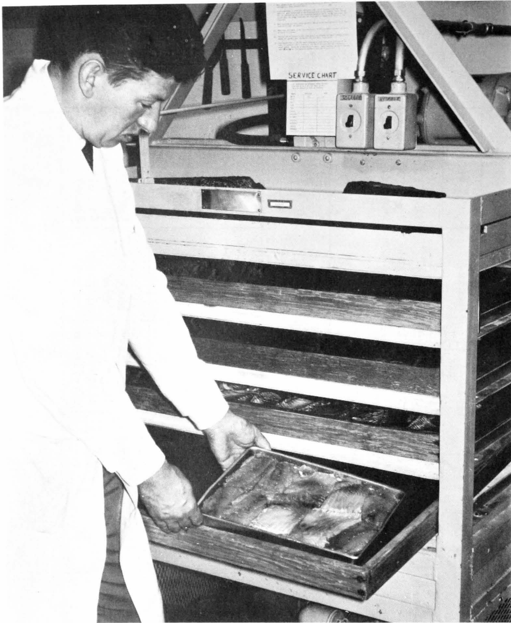
Figure 6.--Freezing blocks of "scored" buffalo loins on a double-contact plate freezer.
