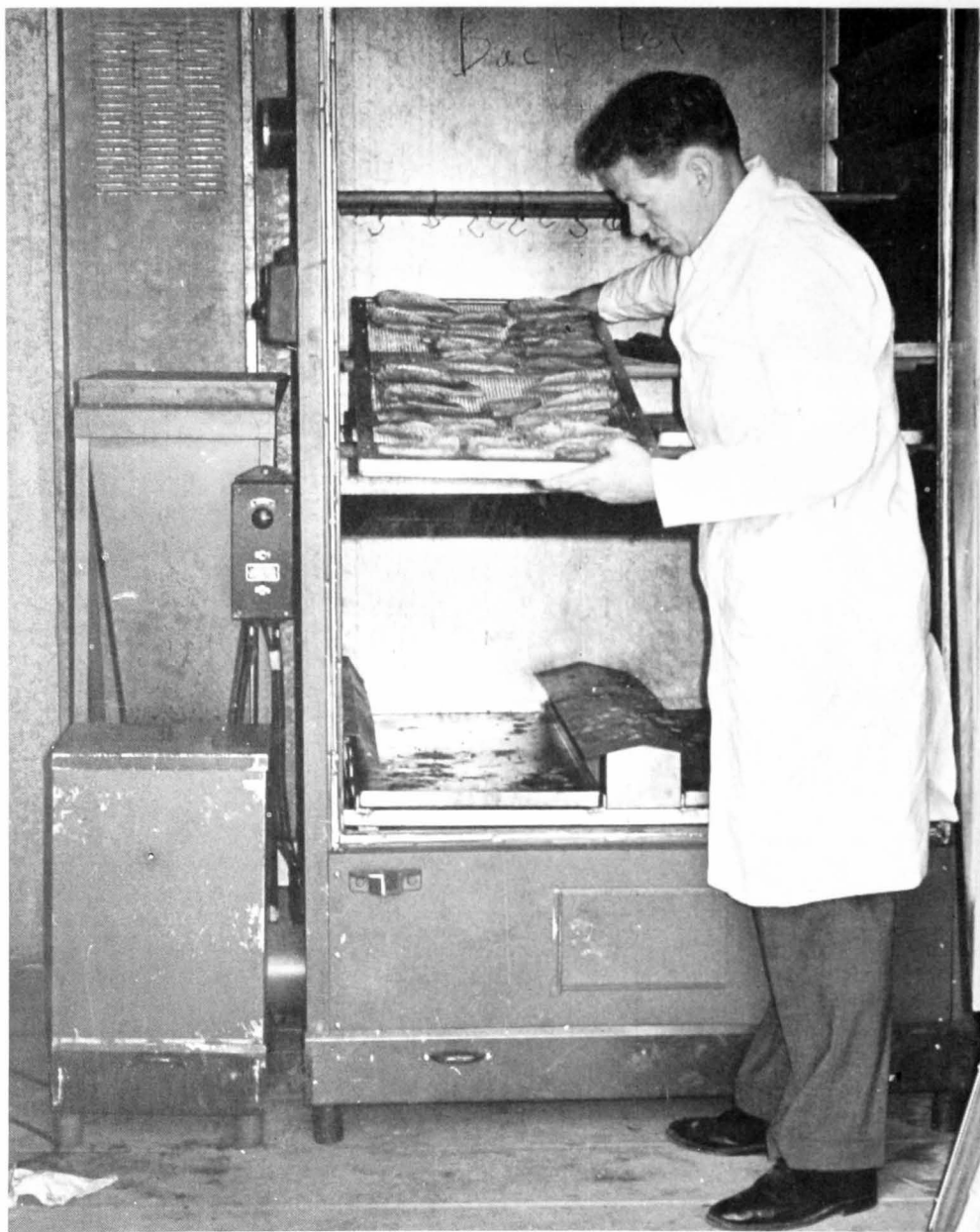
Figure 5.--Smoking buffalo ribs using an electric smokehouse with independent smoke-producing unit.
