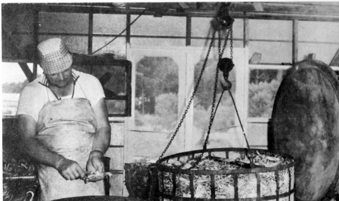
A worker is debacking crabs and scraping out viscera into the drum below. Basket of crabs on the right is cooling.
