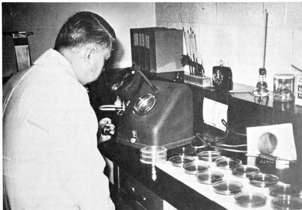
Bacteriologist is determining the standard plate count on dilutions made from samples of freshly picked crab meat. Counter is in his left hand.
