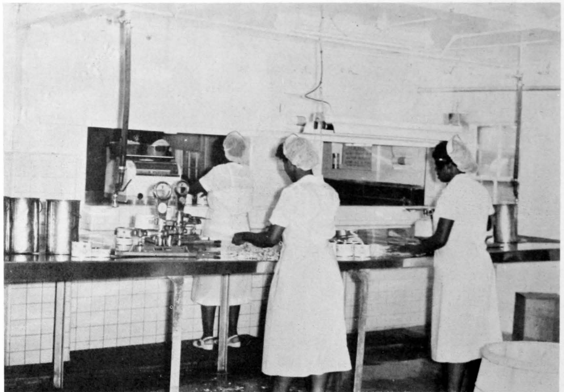
Packing room of another plant in the Chesapeake Bay region. Tile walls and stainless steel tables, scales, etc., make it easy to keep the packing room spotlessly clean.
