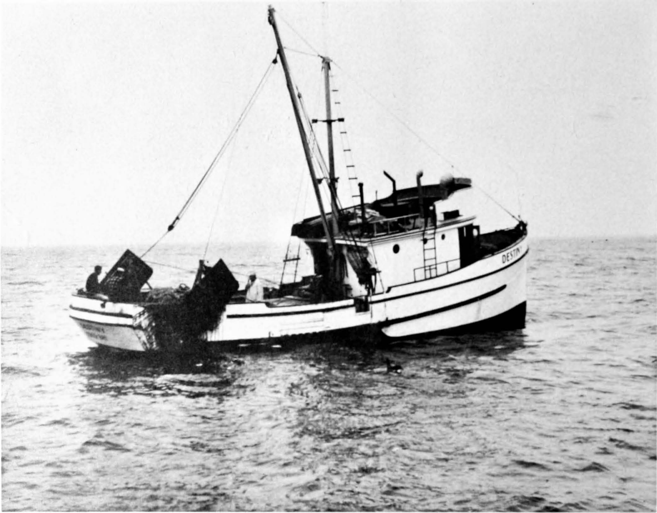
Figure 27.—An otter trawler. Large otter boards on stern are used to open mouth of net, which is dragged on ocean bottom.
