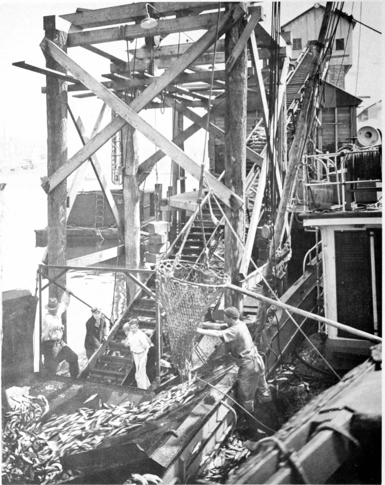
Figure 24.—Brailer used to unload sardines from vessel to conveyor belt at reduction plant in Aberdeen, Washington.
