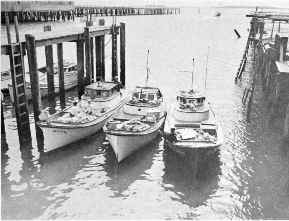
Figure 12.—Typical Columbia River gill-net vessel. Note that the net is hauled from the bow.
