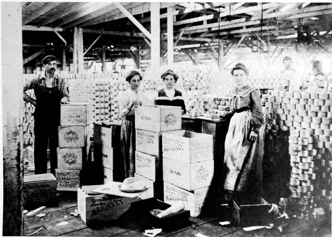
Figure 2.—Warehouse of early salmon cannery where cans were cooled, hand-labeled, and cased.
