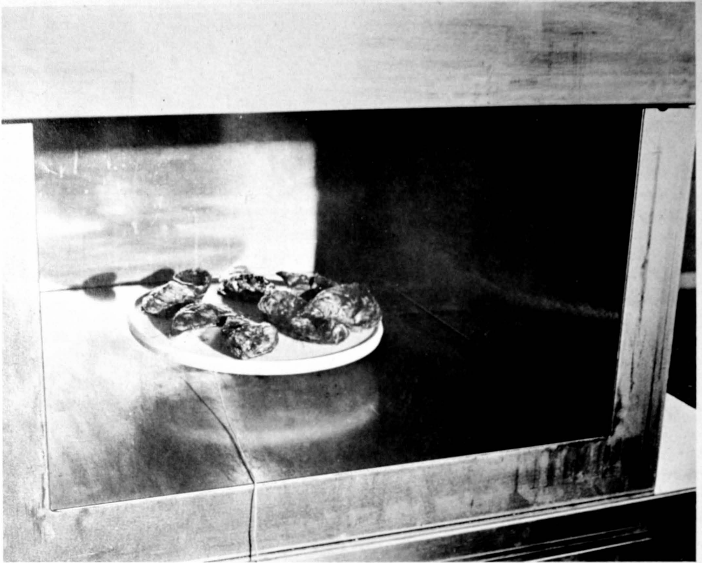
Figure 2.—Oysters on a metal-free turntable inside the oven of the microwave-energy range.
