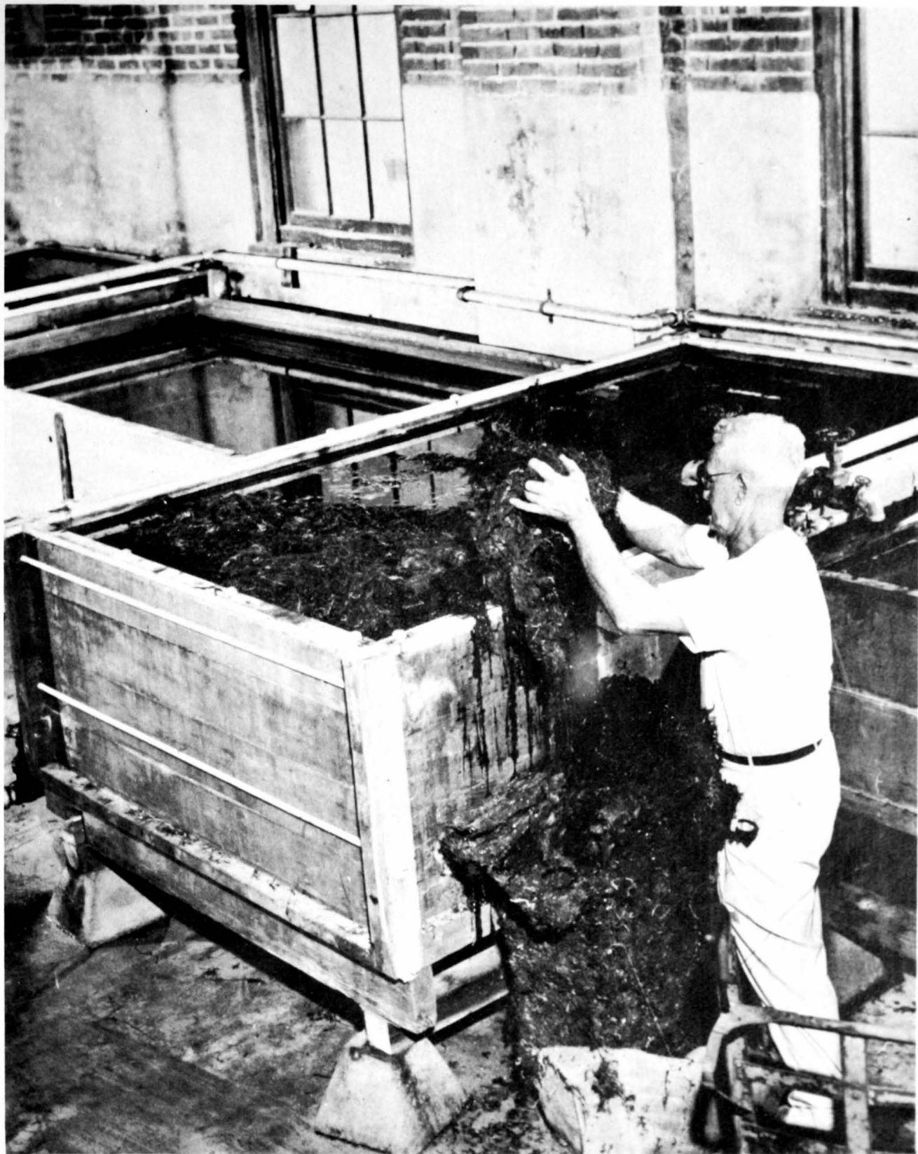
Figure 9.—Seaweed being washed and chemically treated to remove various gums and minerals.
