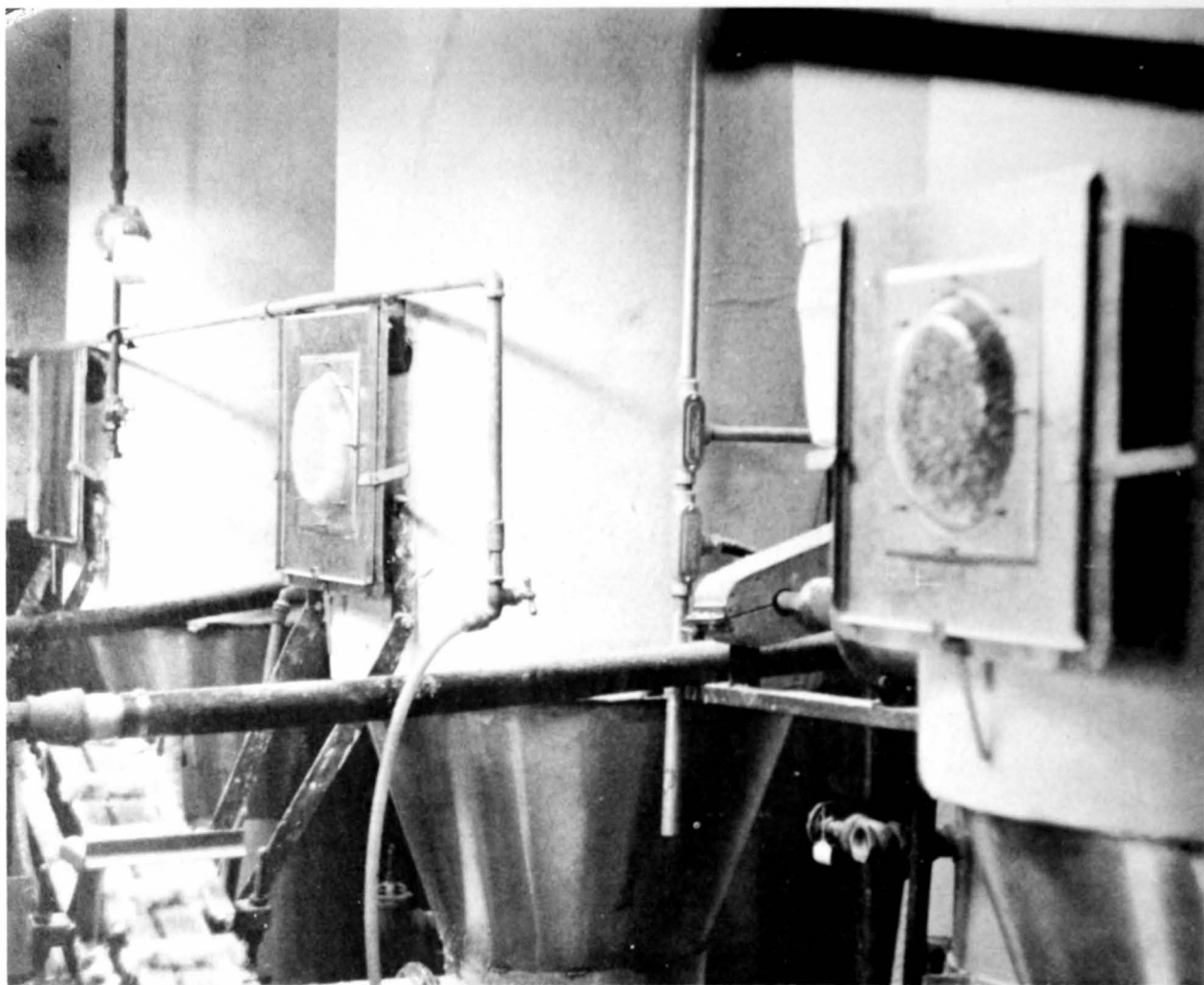
Figure 14.—Removal of water from agar by suction.
