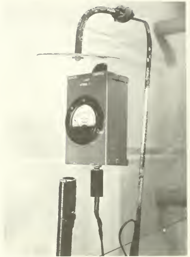
Figure 22.--Underwater remote readout light meter. Underwater detector frame with grey target panel on left and light-cell housing on right. Readout housing in center.
