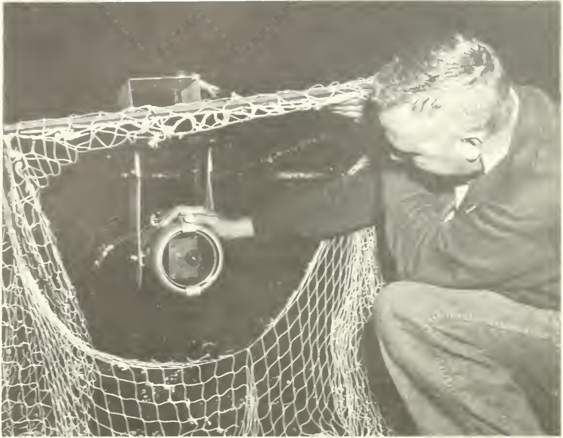
Figure 13.--Front view of plywood-webbing camera mount and small camera. Position of camera in housing is visible.
