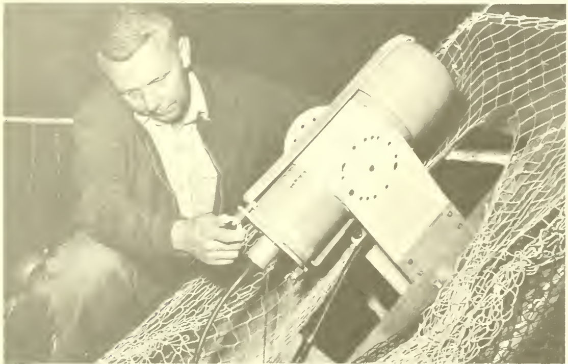
Figure 12.--Plywood-webbing camera mount showing small camera in horizontal position in adjustable aluminum stand. Front closure ring, aluminum closure straps, rear plate, and Joy plug assembly shown.
