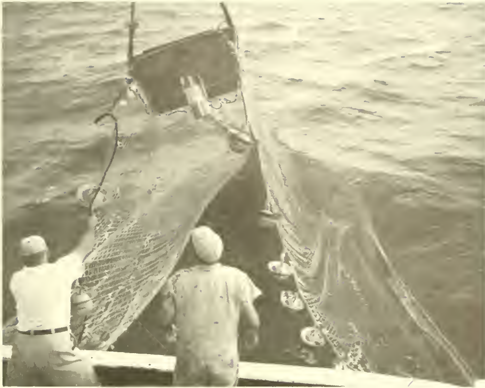
Figure 19.--Small camera on trawl headrope. Metal frame (fig. 2) replaces plywood panel.
