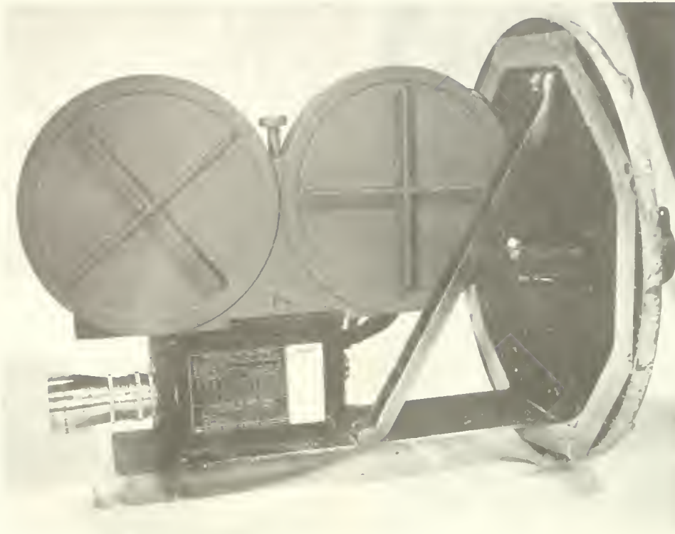
Figure 5.--400-foot film magazine and mounting plate on top of LB-4A magazine. Wire leads from Joy plug are seen on the housing port.
