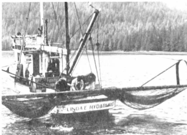
Figure 6.--Beam trawl in operation. Fisherman preparing to release trawl.
