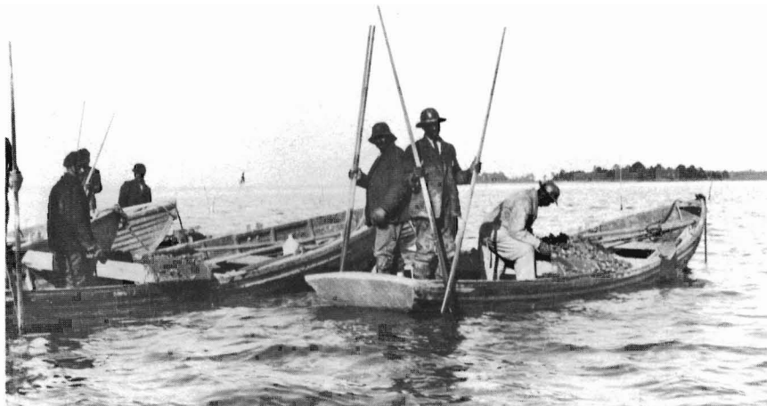
Figure 92.—Tonging oysters in Yankee-designed skiffs in Virginia waters. A crewman propelled the boats by rowing in the bow while standing. Photograph courtesy of the Mariners' Museum, Newport News, Va.
