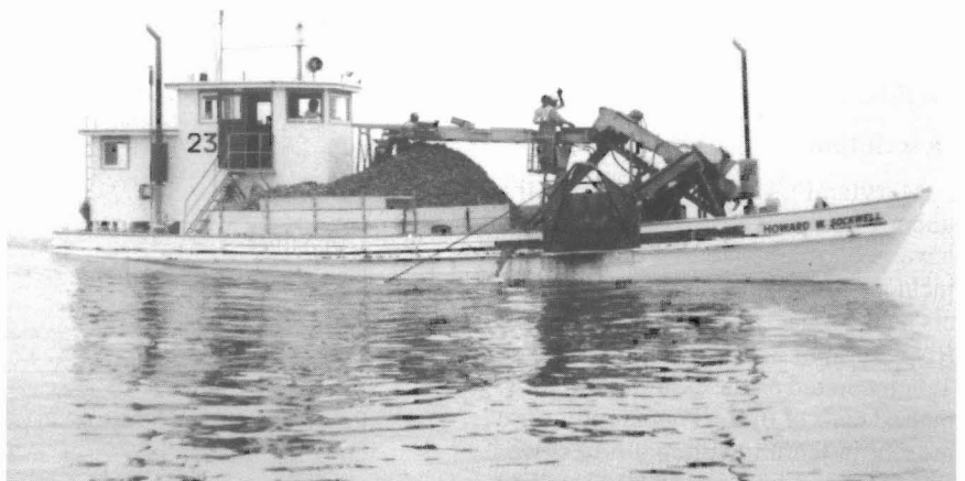
Figure 68.—Above, a New Jersey oyster vessel rigged with relatively new rotary drum for harvesting seed oysters from Delaware Bay. The Cashier , constructed in the 1860's, may be the oldest oyster vessel in the United States. Below is a modern dredging vessel with an automatic dredge dumper.
