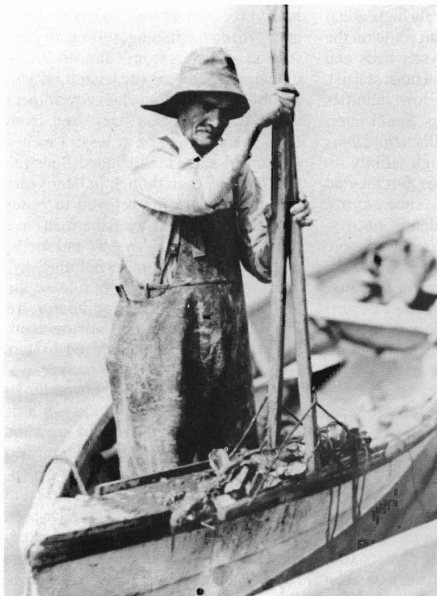
Figure 41.—A fisherman tonging in his dory, which he propelled with oars. Culling board is at the bow, and the tongs have a wooden head, ca. 1920's. Photograph courtesy of the Canadian Department of Fisheries and Oceans, Charlottetown, P.E.I.
