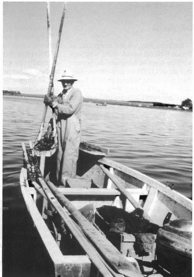
Figure 42.—Modern style oyster "dory" used in Bedeque Bay, propelled by outboard motor. The oysters are held in fishboxes which hold about 1.25 U.S. standard bushels. Photograph by A. Morrison.
