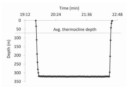
Figure 2.—Plot of the test deployments using 4 kg of lead. Plot illustrates gear sink rates that are sufficient to position hooks below the average thermocline depth in <1 min. Once at the target depth, the gear is maintained at a relatively constant position throughout the deployment period.
