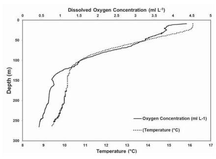
Figure 6.—Depth vs. water temperature (°C) and dissolved oxygen concentration (ml/L) collected during deep-set buoy gear trials off the coast of southern California
