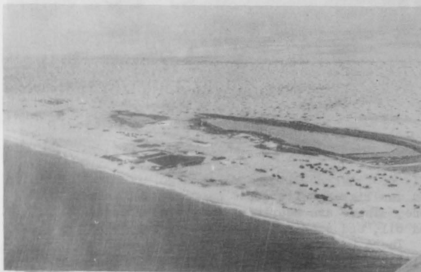
ANGOLAN FISHING VILLAGE NEAR BENGUELA. NOTE EVAPORATION BEDS FOR THE PRODUCTION OF SALT FROM SEA WATER.
