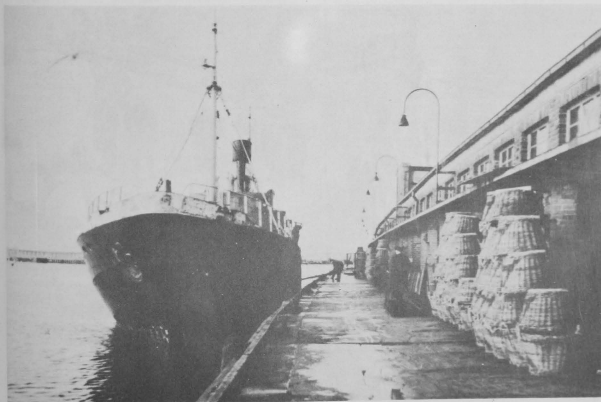
GERMAN TRAWLER ALONGSIDE DISCHARGING QUAY AT AUCTION HALL X, BREMERHAVEN. BASKETS AT SIDE ARE USED TO DISCHARGE FISH AND HOLD ABOUT 50 KG. OF FISH.
