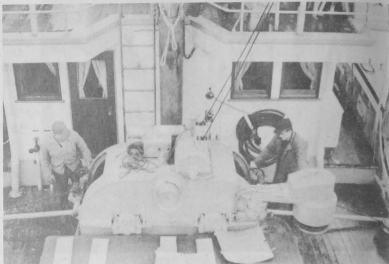
FIGURE 8 - PORTION OF AFTERDECK OF JOHN N. COBB SHOWING TRAWLING WINCH IN OPERATION.
