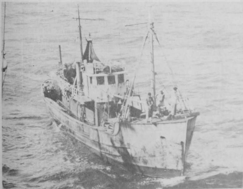
FIGURE 6 - THE TAIRYO MARU NO. 23 (55 GROSS TONS) COMING ALONGSIDE THE TENYO MARU NO. 2 . THIS WAS THE SMALLEST REGULAR LONG-LINE VESSEL PARTICIPATING IN THE EXPEDITIONS.
