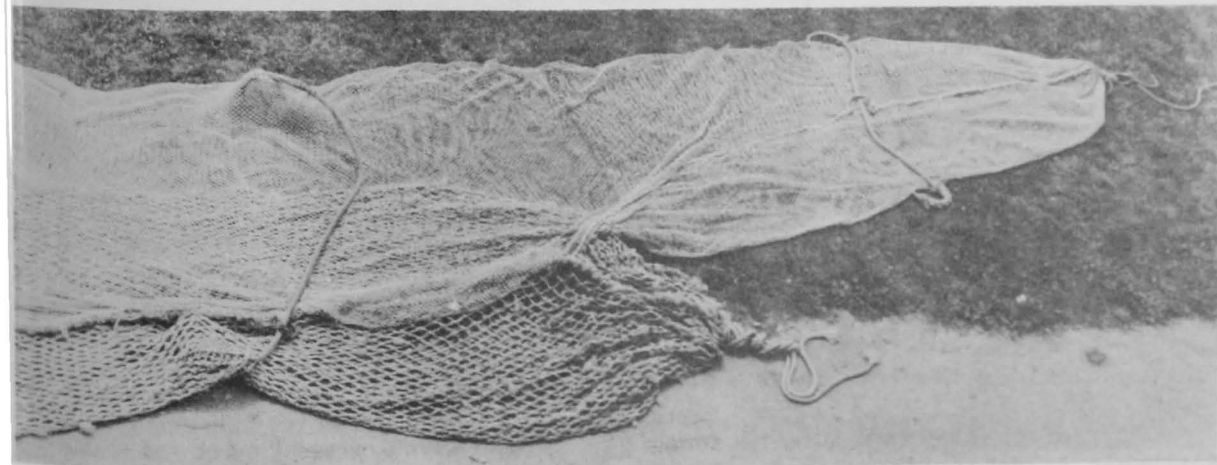
FIGURE 1--FINE-MESHED SHRIMP NET COVER ATTACHED TO UPPER PART OF COD END BEFORE ATTACHMENT OF BULL HIDES.
