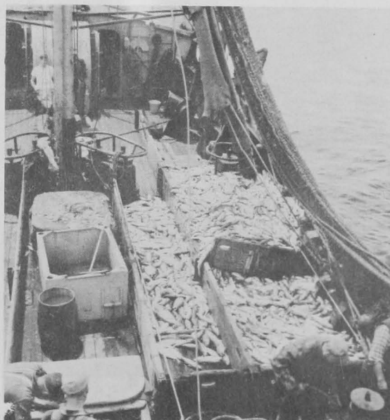
Cod end has been emptied and trawl is again put overboard for another tow.
