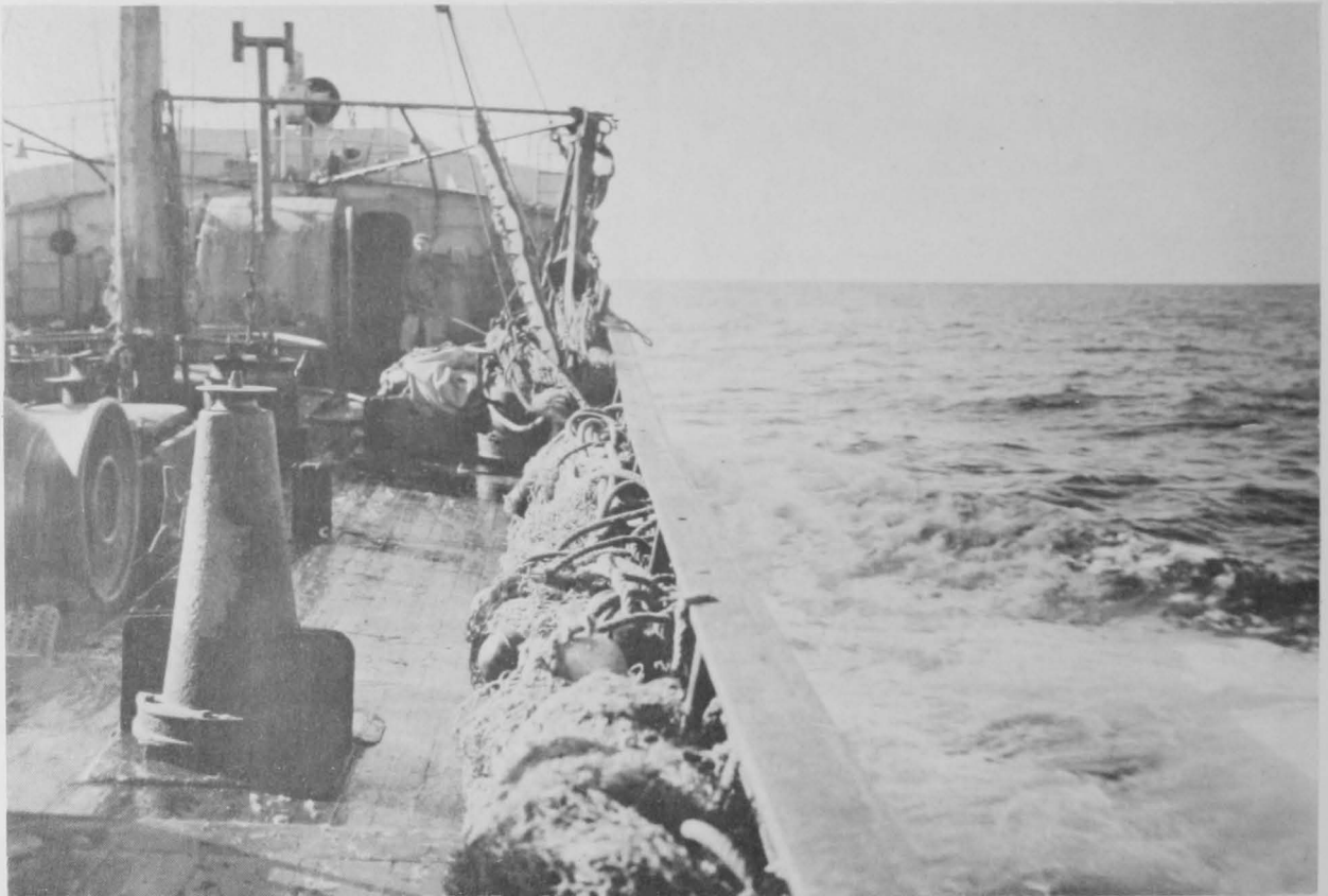
The trawl is secured to the rail of the vessel en route to sea. A duplicate trawl is carried on the opposite side of the vessel. Fishing may be done from either side.
