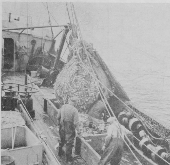
The cod end or bag of fish is hoisted aboard. A fisherman releases drawstring at bottom of bag to discharge fish on deck.
