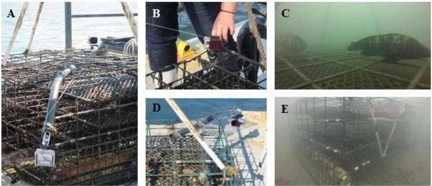
Figure 2. On bottom cage with camera views. (A) Close-up of cage fitted with cameras, showing side view in the front of the photo and top camera at the rear. (B) Close-up of top camera looking across the horizontal surface of the cage. (C) The resulting view of the top camera. (D) View of the side camera looking at two sides of the cage and where the cage meets the sea floor. (E) Resulting view of the side camera.
