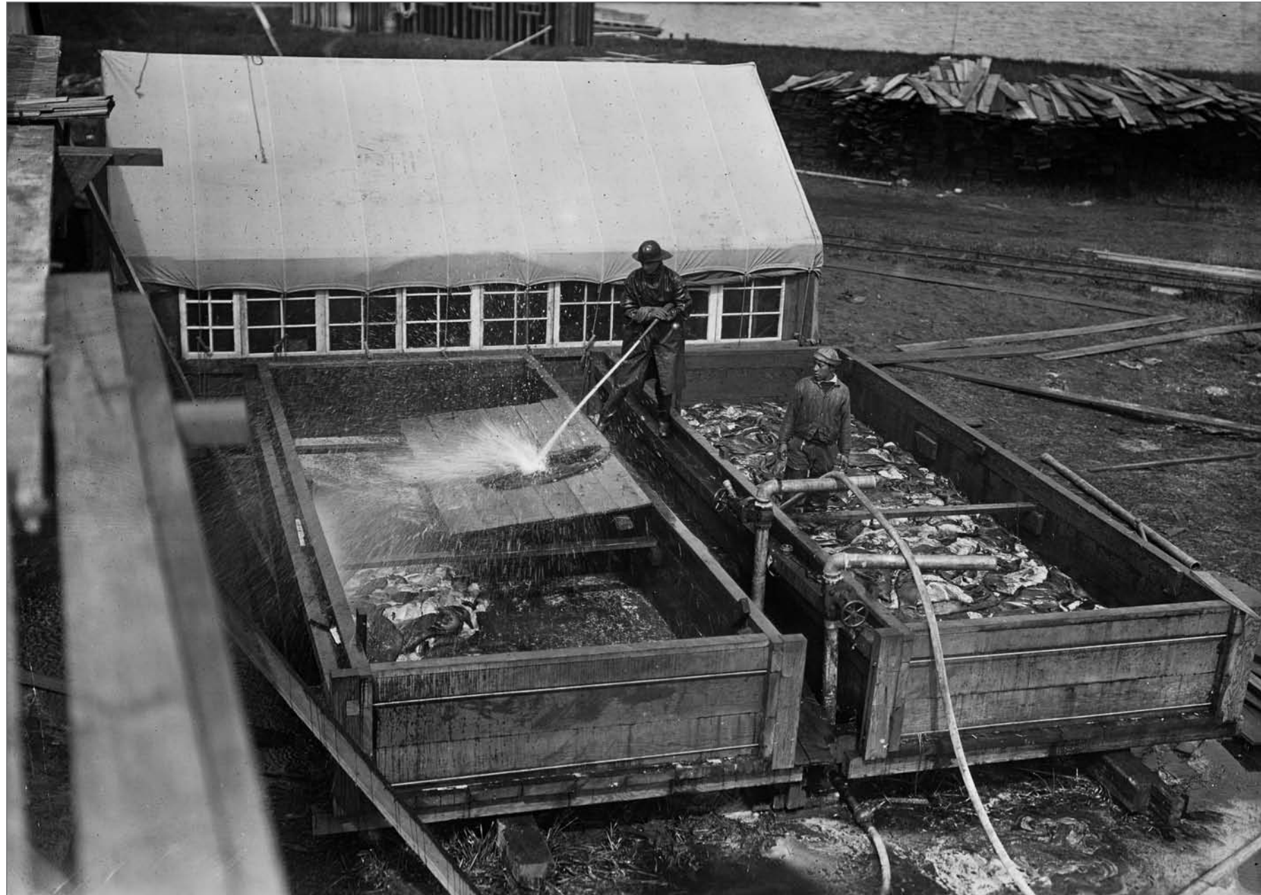
Photograph No. 95-ADMC-585 (Photographer unknown), 1921; Men hosing sealskins in wash tanks to remove dirt and blood prior to blubbering. Records of the National Oceanic and Atmospheric Administration, RG 370; NARA—Pacific Alaska Region (A).
