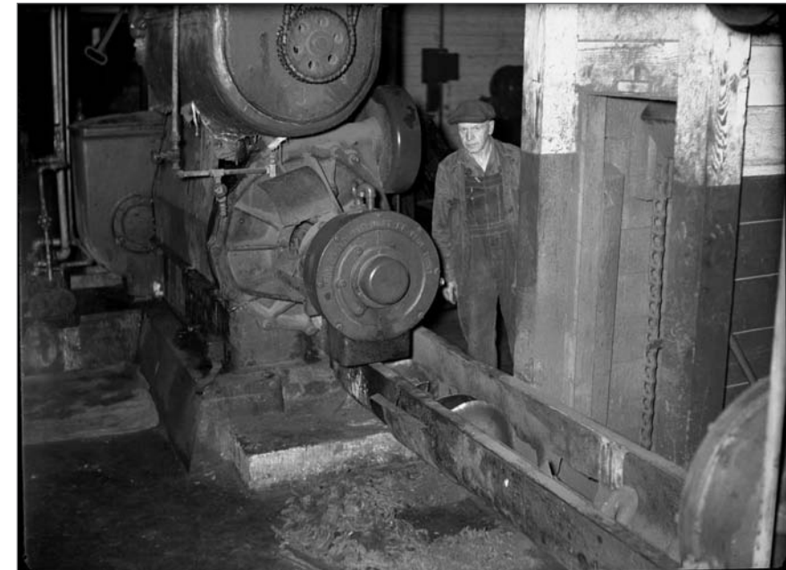
Scheffer, Victor B., photographer. 1947. "By-products plant, St. Paul Island, Alaska, 24 July 1947. Expeller where oil is pressed from cooked seal meal. The meal moves toward the shaft (right side) and goes up to the left." Photograph. NOAA, NMML Library, Seattle: Victor B. Scheffer Collection, Fur-Seal Archives, neg. no. 2234.
