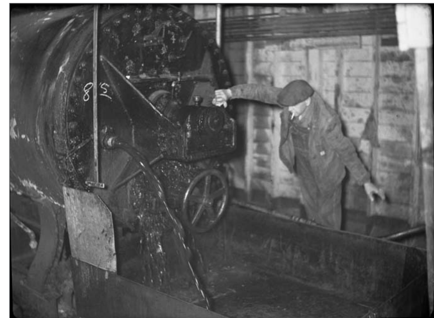
Scheffer, Victor B., photographer. 1947. "By-products plant, St. Paul Island, Alaska, 24 July 1947. Releasing blubber oil, after 3 hours at 380 lbs. [pressure]." Photograph. NOAA, NMML Library, Seattle: Victor B. Scheffer Collection, Fur-Seal Archives, neg. no. 2233.
