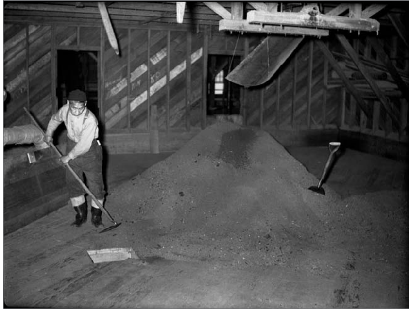
Scheffer, Victor B., photographer. 1947. "By-products plant, St. Paul Island, Alaska, 24 July 1947. Loft, with seal meal piling up. At intervals, it is pushed through a hole in the floor to the hammer mill." Photograph. NOAA, NMML Library, Seattle: Victor B. Scheffer Collection, Fur-Seal Archives, neg. no. 2235.
