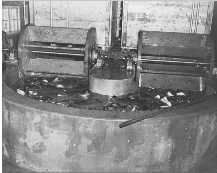
Photograph No. 95-ADMC-928 (Photographer unknown), n.d.; 5,000-gallon concrete oval brining tank for curing fur sealskins, constructed on St. Paul Island. Records of the National Oceanic and Atmospheric Administration, RG 370; NARA—Pacific Alaska Region (A).
