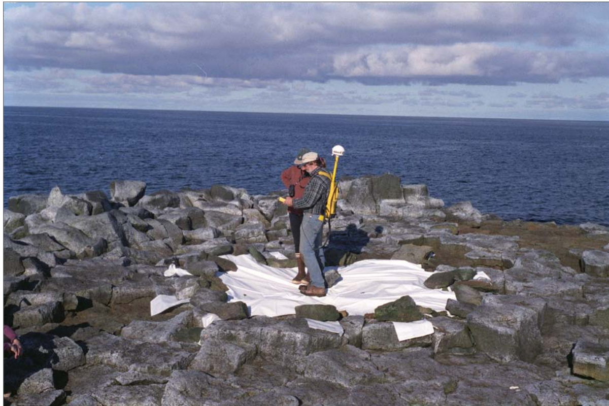
GIS crew on Walrus Island, showing geo-referencing marker, spring, 2001. Photograph. NOAA, NOS, Pribilof Project Office, Seattle.
