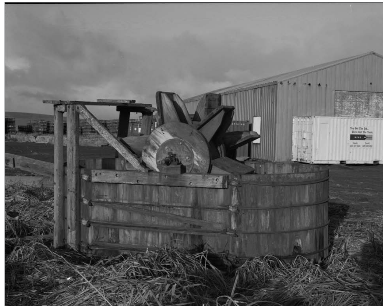
Lindsay, John A., photographer. 2001. Redwood brine tank used in the Wash House on St. Paul Island to wash sealskins. The tank was moved to a site at the airport. It was damaged during snow plowing during 2007. Photograph (6x7cm). NOAA, NOS, Pribilof Project Office, Seattle: sheet JL110930.3, neg. 3819.
