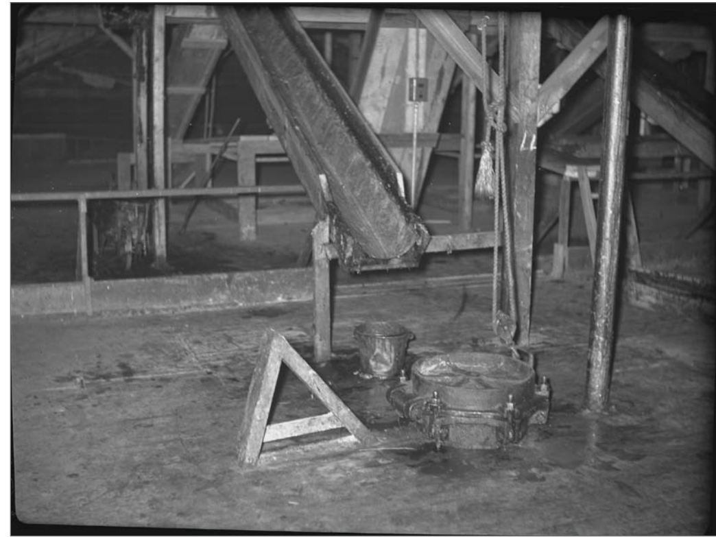
Scheffer, Victor B., photographer. 1947. By-products Plant. Chute where chopped seal meat enters cooker mouth, July 24, 1947. Photograph. NOAA, NMML Library, Seattle: Victor B. Scheffer Collection, Fur-Seal Archives, neg. no. 2243.
