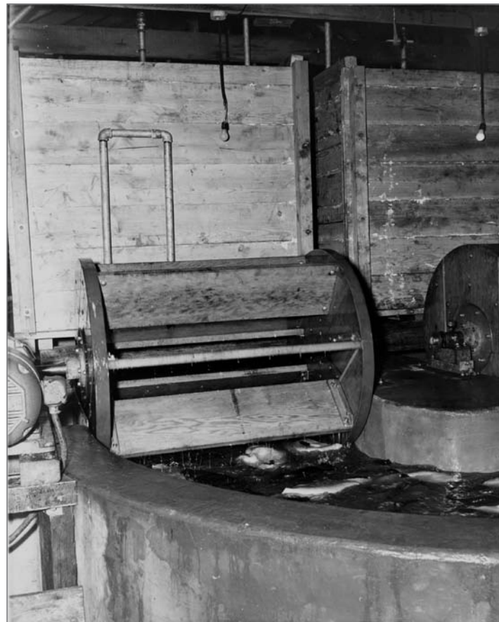
Photograph No. 95-ADMC-895 (Photographer unknown), 1953; Paddles in 5,000-gallon capacity brining tank. Records of the National Oceanic and Atmospheric Administration, RG 370; NARA—Pacific Alaska Region (A).
