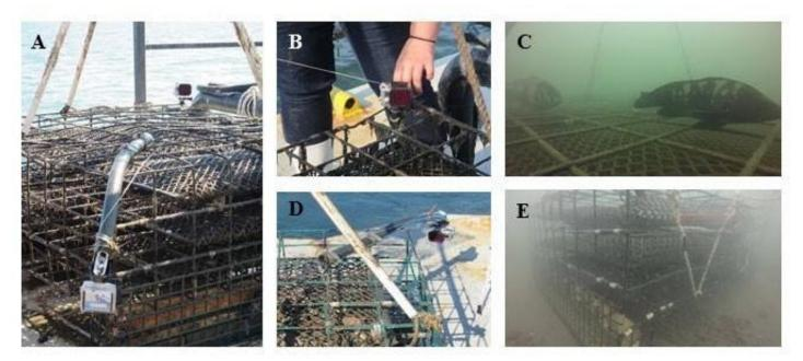
Figure 2. On bottom cage with camera views. (A) Close-up of cage fitted with cameras, showing side view in the front of the photo and top camera at the rear. (B) Close-up of top camera looking across the horizontal surface of the cage. (C) The resulting view of the top camera. (D) View of the side camera looking at two sides of the cage and where the cage meets the sea floor. (E) Resulting view of the side camera.
