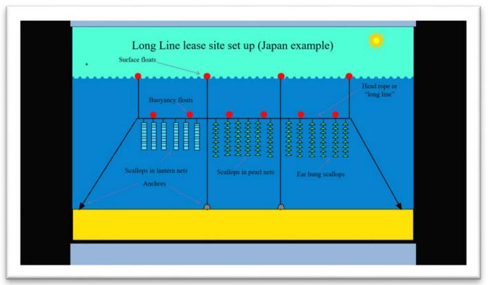
Figure 4. Schematic of a typical longline.
