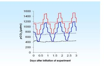
Figure 1. Changes in partial pressure of  $CO_2$  in experimental seawater during the diel cycle treatment experiment conducted 21-24 December 2010 in the Shiogama laboratory. Lines represent the values monitored by the AICAL system every hour. Dotted lines represent values in the constant treatment (1200, 800, 450 (atmosphere balanced)  $\mu$ atm) and line represents those in the diel cycle treatment (400-1200, 800-1600  $\mu$ atm), respectively.
