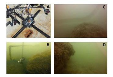
Figure 3. T-platform construction to mimic camera views on natural structured habitat. (A) Full view of t-platform with cameras attached. (B) Image of t-platform deployed on a natural rock reef adjacent to boulder. (C) Resulting top view of the boulder. (D) Resulting side view of the boulder which also captures where the boulder and sea floor meet.
