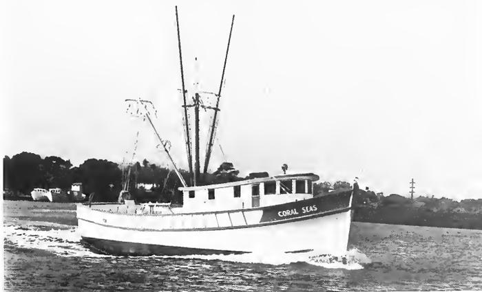
The Coral Seas (67 gross tons, 62 feet long, 333 horsepower) was built in 1966 for Charles J. Kiesel and Hilbert J. Kiesel, Fort Myer, Fla. This vessel is typical of the new wooden hull vessels constructed for shrimp fishing.
