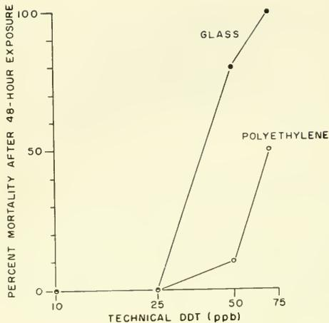
Tests of DDT on pinfish, Lagodon rhomboides in 40-liter volumes showing that toxicity was reduced by use of polyethylene bags for containers over use of glass vessels.
