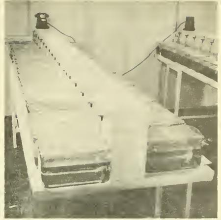
Glass jars which have replaced polyethylene vessels used in bioassay of pesticides. Four to six concentrations of each compound are tested simultaneously. Jars at left are used for fish, each holding 40 liters of medium and 10 specimens. Because of cannibalism, shrimp and crabs require isolation. Individual animals are held in 4 liters of medium in smaller containers (right), 10 being required for each concentration tested.
