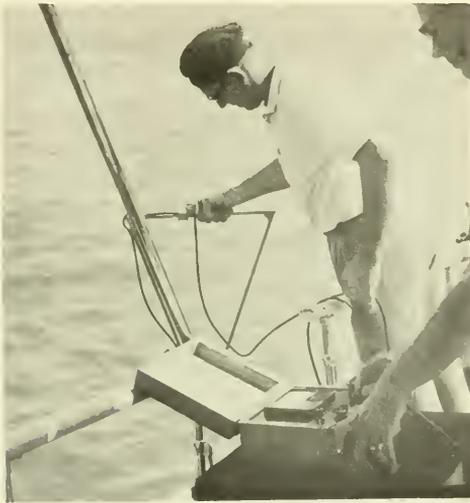
Measuring light intensity with a photocell.
