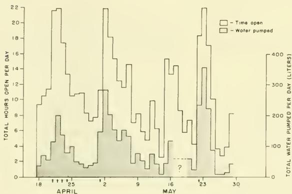
Daily record of number of hours open and volume of water pumped by an oyster maintained in sea-water laboratory. Because of failure in the experimental set-up no record of volume of water pumped was obtained on May 17, 18, and 19. Arrows indicate the dates that some fresh sea water was added to the system.
