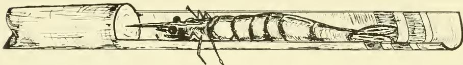
Device for rapid measurement of small shrimp. Basic construction is of plastic tubing. Note variously colored size-range calibrations.
