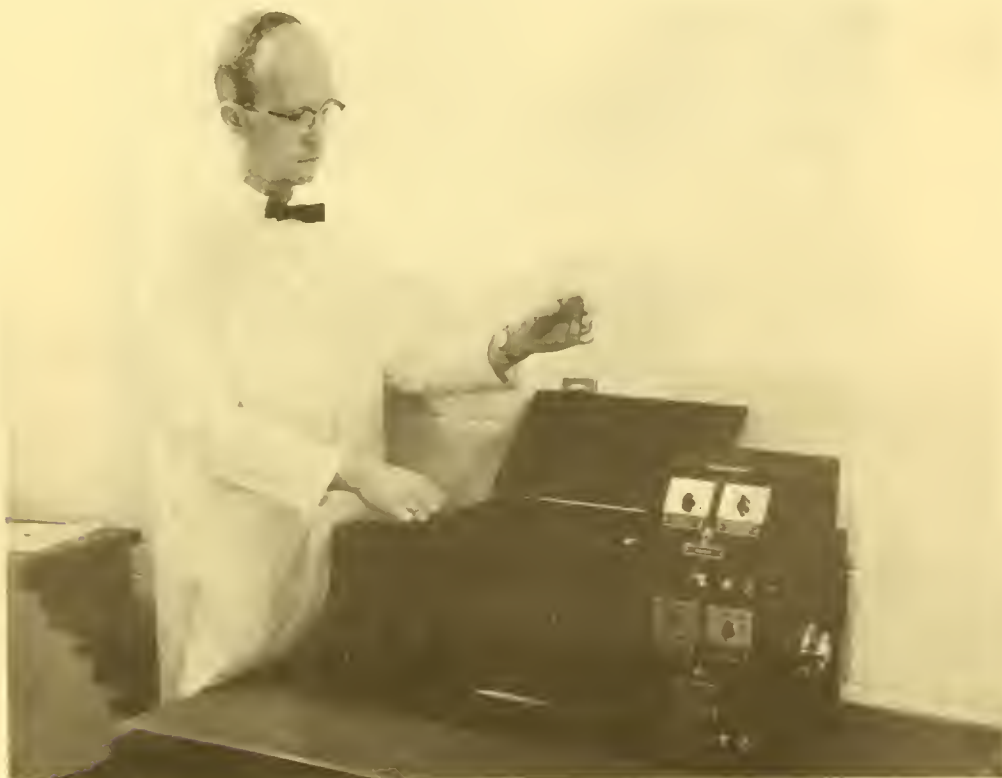
Making light-scattering measurements to determine the effect of frozen storage on the size and shape of actomyosin molecules from cod muscle.
