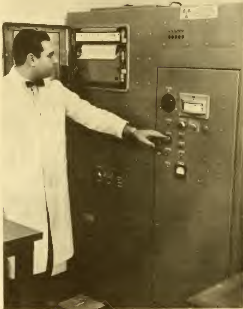
Using the gas chromatograph for the separation of volatile compounds that contribute to the odor and flavor of fresh haddock.
