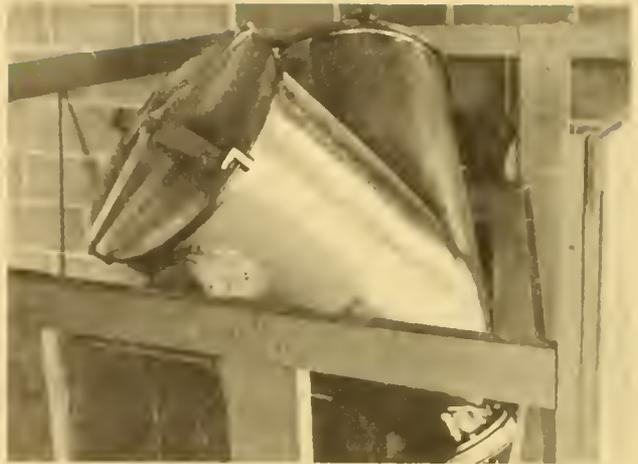
Y-shaped rotary blender used for mixing diets containing pesticide.
