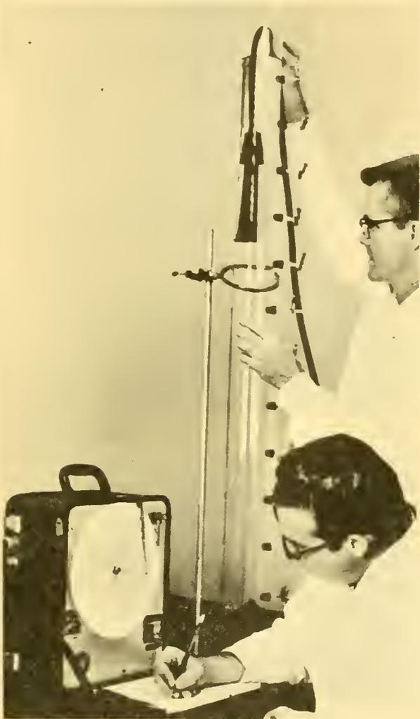
Determining salinity gradient with conductivity meter.
