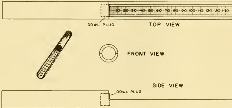
Shrimp measuring device made of plastic tubing.
