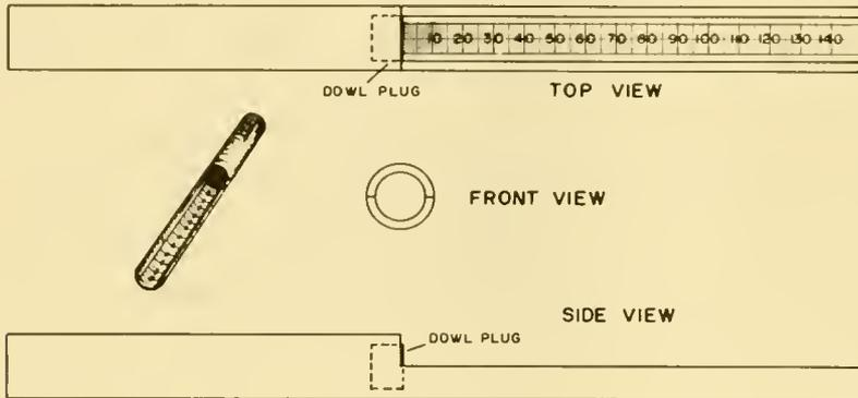
Shrimp measuring device made of plastic tubing.
