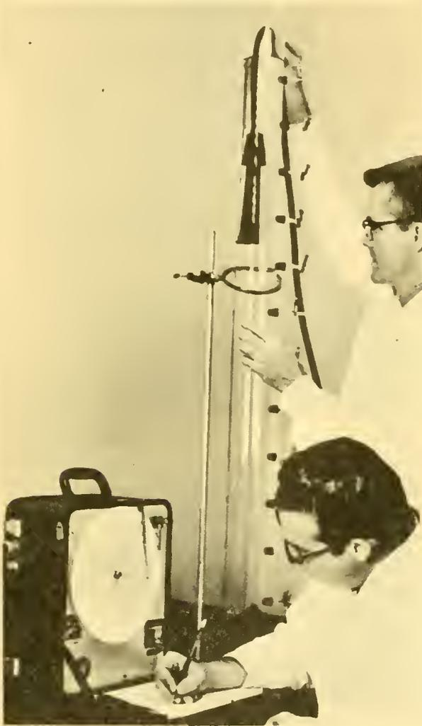
Determining salinity gradient with conductivity meter.
