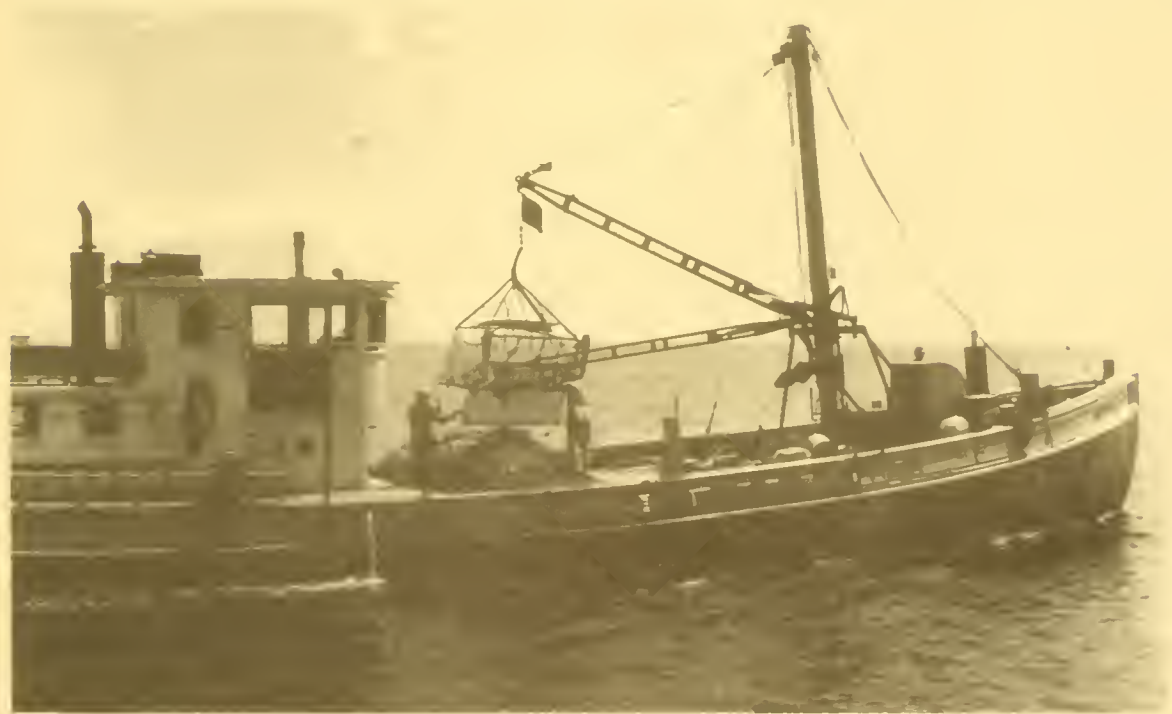
Figure 23.--Modern type of oyster dredge which is easily unloaded by opening its bottom.
