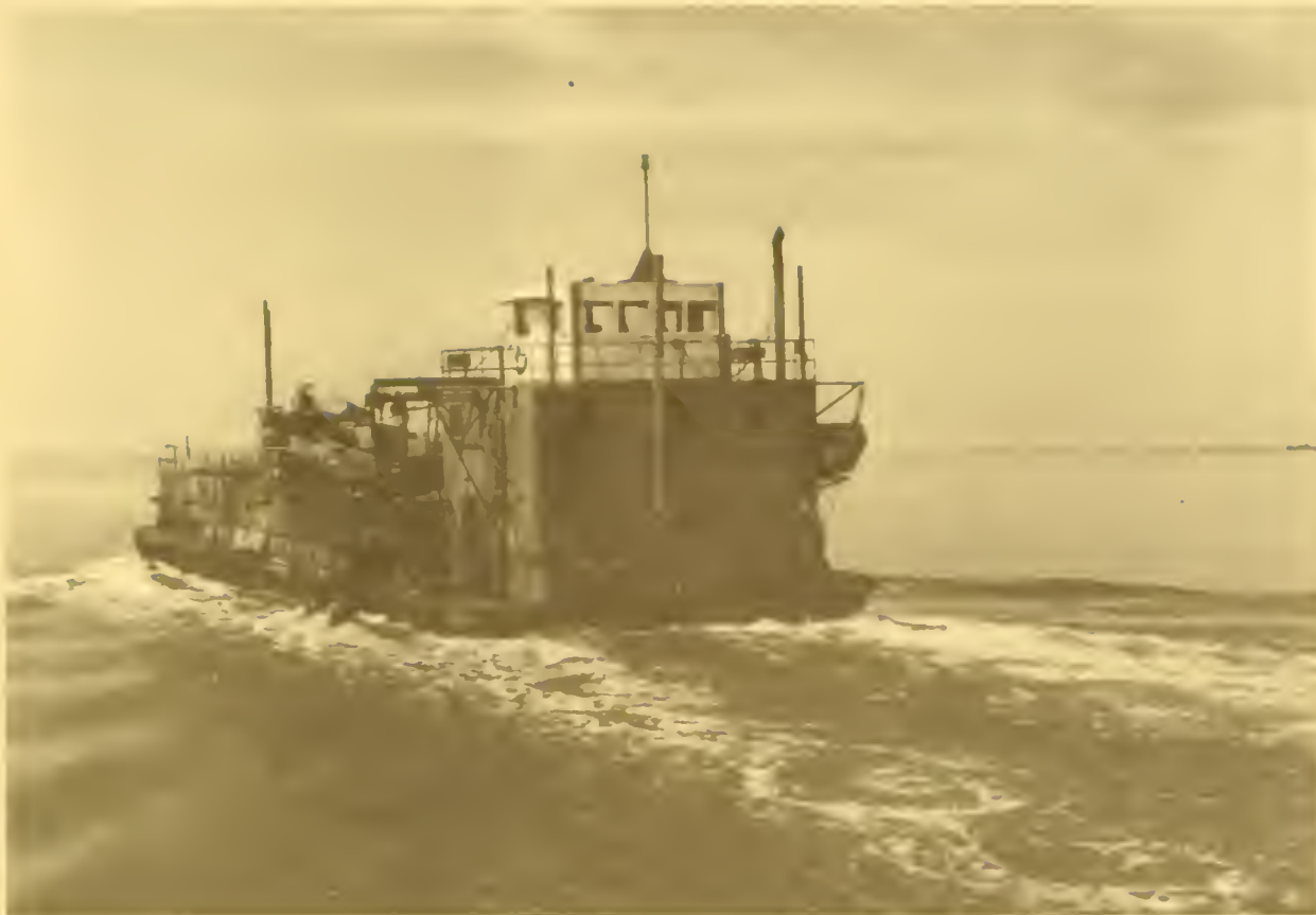
Figure 25.--Large suction dredge operating on oyster beds in Long Island Sound and in the waters of the State of New York. Description in text.
