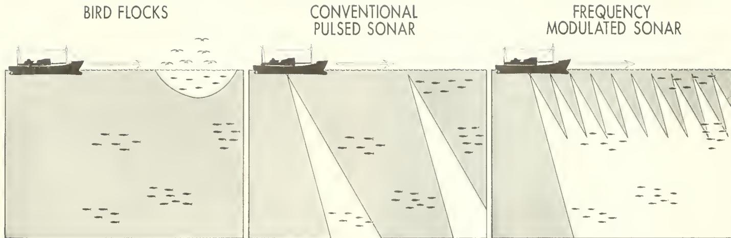
**FIGURE 7.** The new continuous-transmission, frequency-modulated sonar to be installed aboard the *Townsend Cromwell* will allow scientists to track individual fish and fish schools underwater. To locate tuna schools the commercial fleet now depends heavily on sighting bird flocks,
