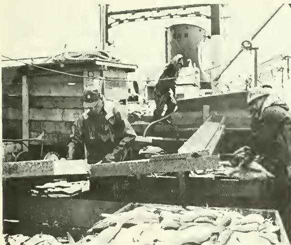
Salmon being cleaned aboard a Japanese factory ship. After being weighed, the salmon are graded and put into bins. The better quality salmon are frozen whole, and the remaining fish are cleaned (gutted and gilled) and canned.
