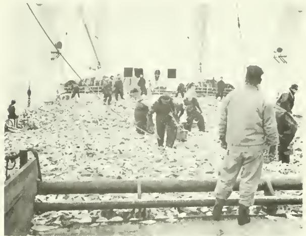
The larger sole and other desirable species of fish being selected from tons of groundfish on deck of a Japanese factory ship in the eastern Bering Sea. The selected fish are frozen for human consumption, and the remaining mass of fish are reduced into meal and oil or made into minced fish meat.
