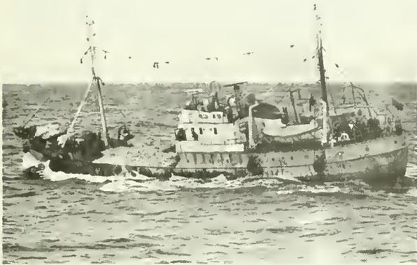
Soviet SRTR side trawler with deck load of ocean perch in Gulf of Alaska. Although this class of side trawler has freezing capabilities, catches are generally delivered directly to accompanying processing vessels.
