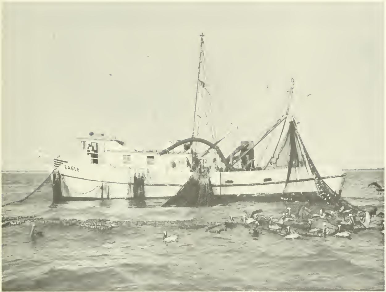
Figure 15.--Single-boat-rig purse seiner used in thread herring fishery.
