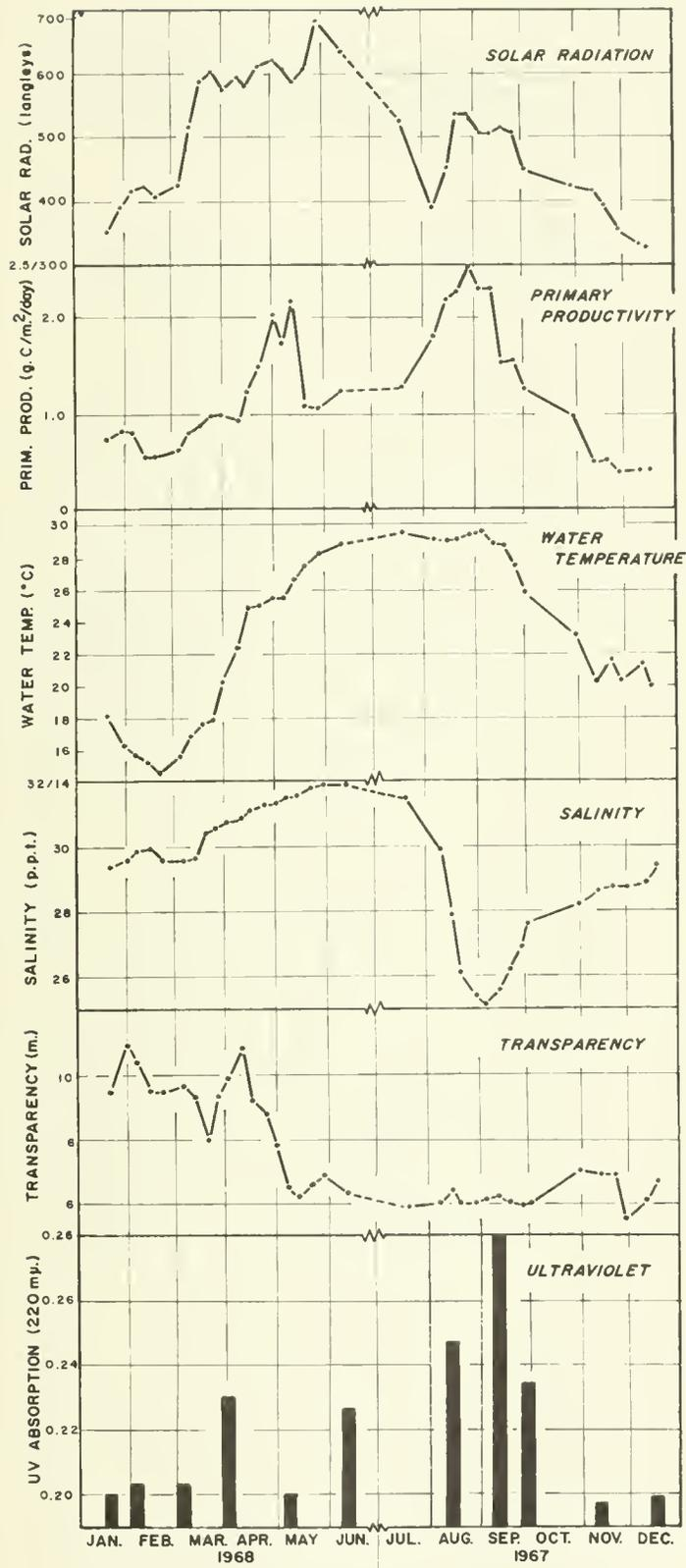
Figure 18.--Comparison of selected properties of the environment in fiscal year 1968. Moving averages of the order three were used to smooth the data except for ultraviolet absorption--for it, raw data were used. Transparency is the depth (m.) to which 35 percent of surface light penetrated. Dashed lines indicate discontinuity between June 1968 and July 1967.
