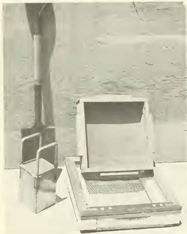
Figure 9.--Benthic sampling equipment: plug sampler and shovel, sieve box, and styrene plastic frame to support sieve box.
