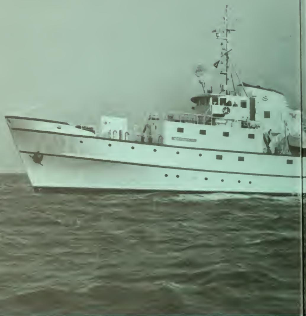
The *Albatross IV*, commissioned in May 1963, was especially designed for fishery-oceanographic research in the northwestern Atlantic. This 187-foot steel stern trawler is equipped with special fishing gear and modern electronic devices including a
