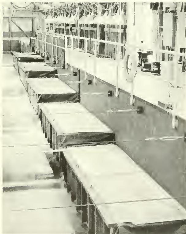
Figure 19.—Covered fishway used in darkened passage experiments. All laboratory lights were turned off during dark tests.
