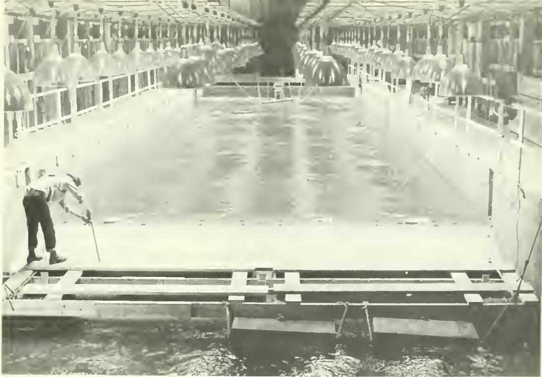
Figure 21.—Experimental arrangement for examining reactions of salmon fingerlings to overfalls and orifices. Approach channel is 24 feet wide and 15 feet deep. Release box may be seen at the far end of the channel. Inclined plane screen trap is visible in the foreground.
