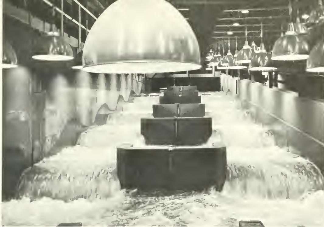
Figure 23.—Ice Harbor design fishway in operation.
