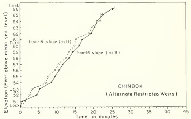
Figure 14.—Pattern of ascent in the 1-on-8- and 1-on-16-slope endless fishways after rest areas were removed from turn pools and with restricted overfalls in the 1-on-8-slope fishway.
