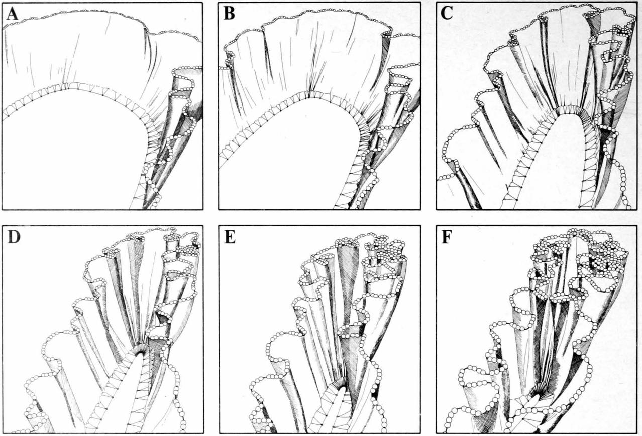
Figure 10.—Successive net configurations assumed by Model II during pursing. (Elongate form assumed as pursing progresses is due to pursing from stationary edge of pool. In practice, drawing of the purse seiner toward center of net during pursing, gives a more circular shape.)
