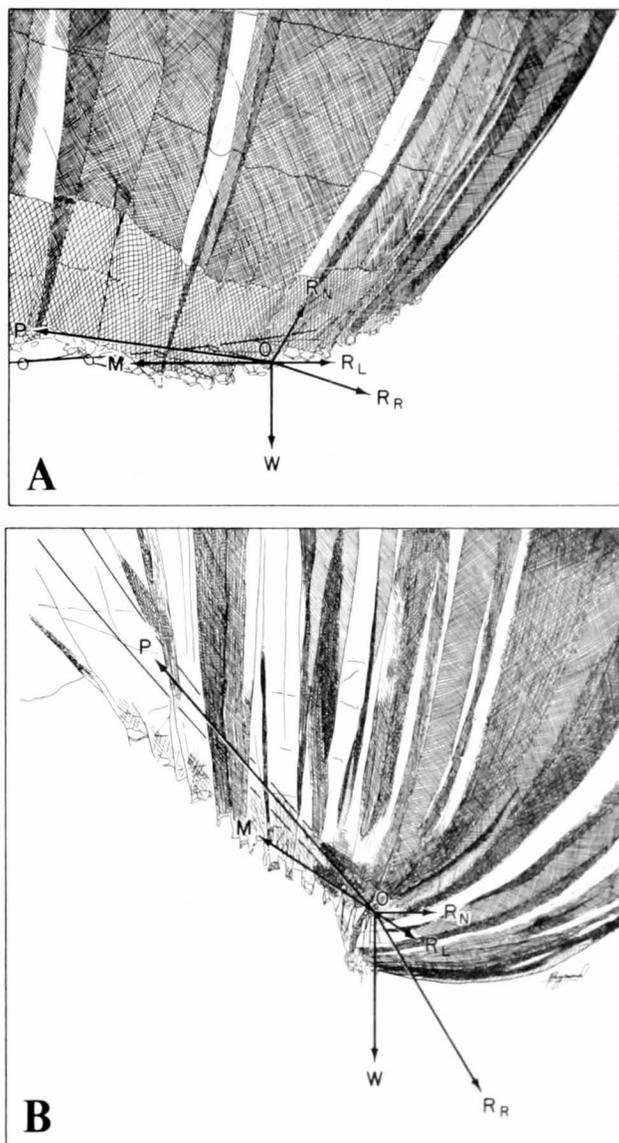
Figure 5.—Pursing forces acting on leadline of Model II: (A) at start of pursing and (B) near completion of pursing. Symbols: O = point of leadline at which forces act. Force vectors: P = pull in purse line,  $R_N$  = pull in netting,  $R_L$  = water resistance on leadline, W = force of gravity. Resultants:  $R_R$  = resultant of  $R_N$ ,  $R_L$ , and W, M = resultant of all forces.
