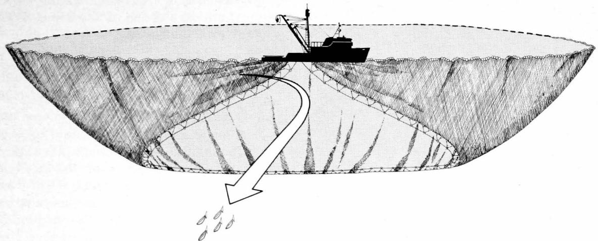
**Figure 14.—Fish escape because of unfavorable configuration of partially pursed net.**
