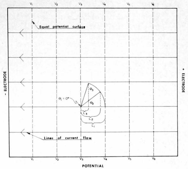
Figure 1.—Uniform electric field showing hashed lines of equal potential surfaces, solid lines of current flow, angle of theta, and the relation between L length of an object at various angles of theta and lines of equal potential ( $V = \text{voltage}$ ).
