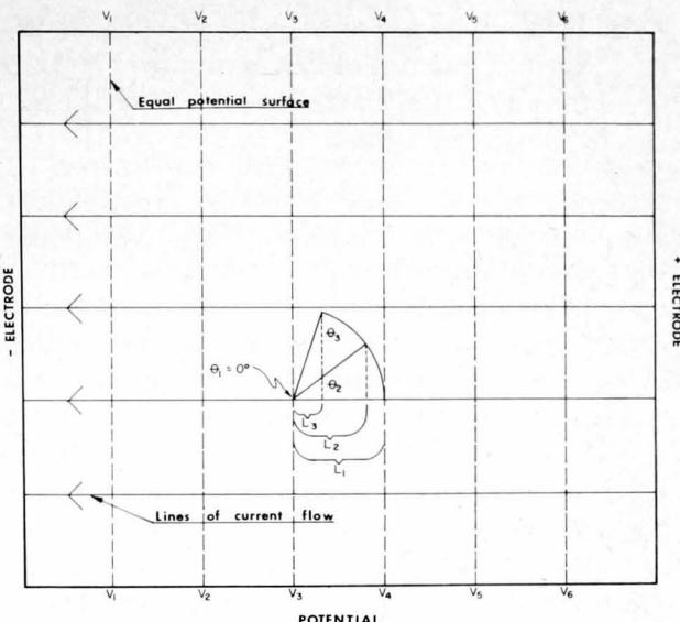
Figure 1.—Uniform electric field showing hashed lines of equal potential surfaces, solid lines of current flow, angle of theta, and the relation between  $L$  length of an object at various angles of theta and lines of equal potential ( $V$  = voltage).
