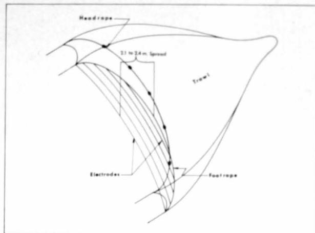
Figure 3.—Diagram of shrimp trawl rigged with the electric system, showing terms used.
