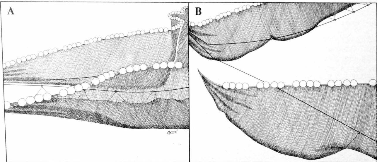
Figure 6.—Wing ends of both models (traced from projected photo transparencies): (A) Model I and (B) Model II.
