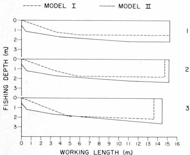
Figure 8.—Approximate shape of one-half the netting of Models I and II at three stages during set:
