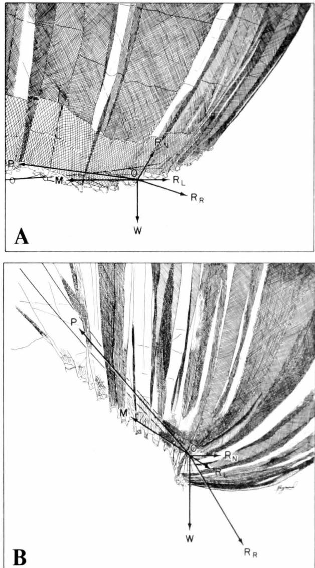
Figure 5.—Pursing forces acting on leadline of Model II: (A) at start of pursing and (B) near completion of pursing. Symbols: O = point of leadline at which forces act. Force vectors: P = pull in purse line, R<sub>N</sub> = pull in netting, R<sub>L</sub> = water resistance on leadline, W = force of gravity. Resultants: R<sub>R</sub> = resultant of R<sub>N</sub>, R<sub>L</sub>, and W, M = resultant of all forces.
