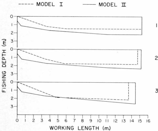
Figure 8.—Approximate shape of one-half the netting of Models I and II at three stages during set: (1) just after completion of circle, (2) just after start of pursing, and (3) pursing one-third completed.
