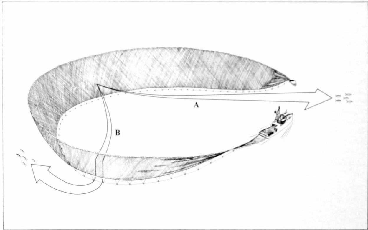
Figure 13.—Fish escape because of (A) inadequate setting speed or judgment errors or (B) net's inadequate sinking speed.
