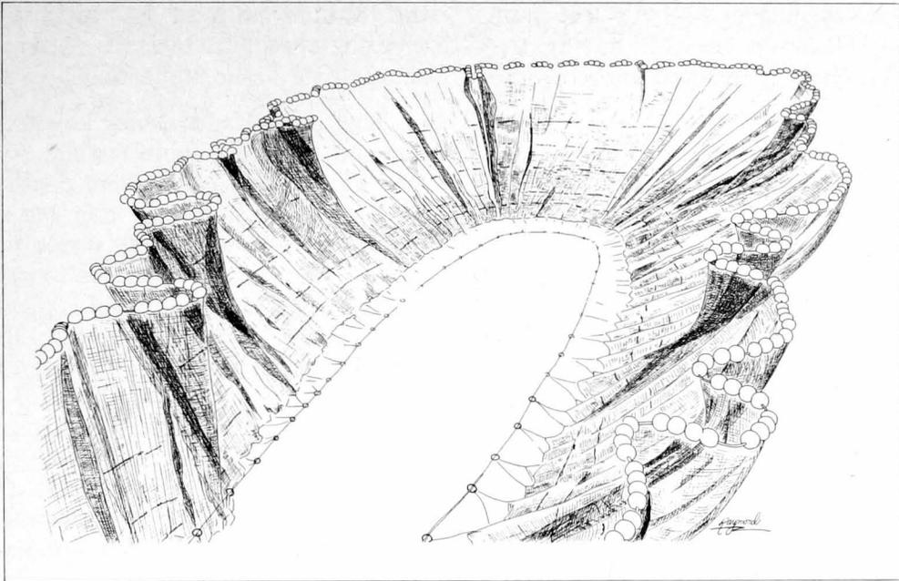
Figure 12.—Scooping action of Model II's leadline (traced from projected photo transparency).
