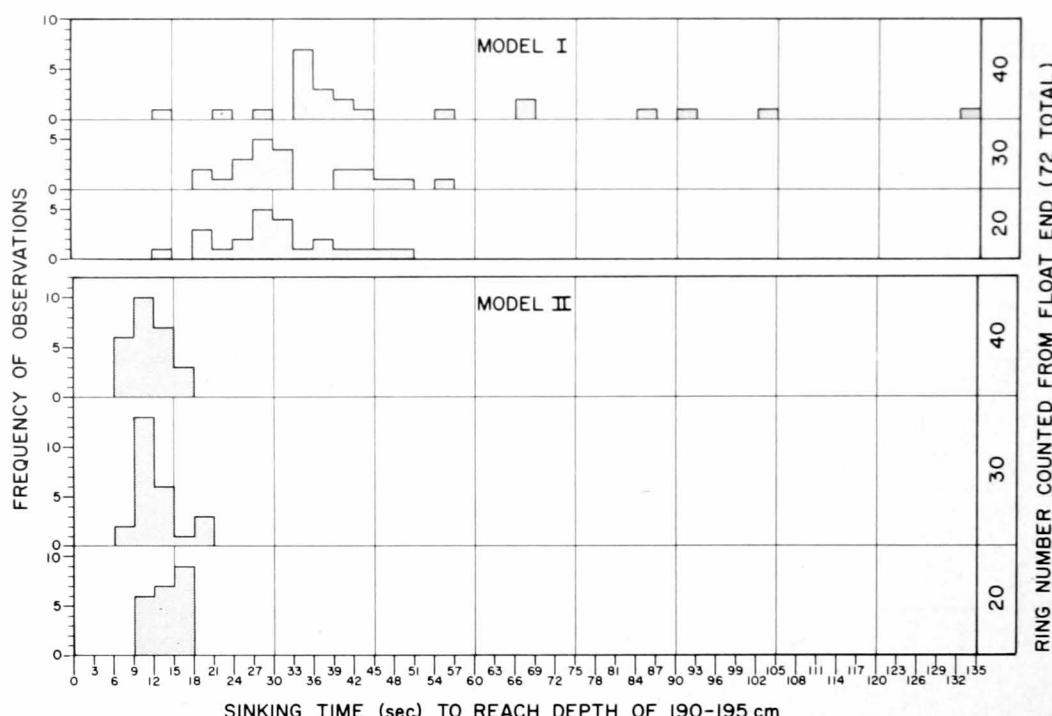
Figure 4.—Sinking time of models.
