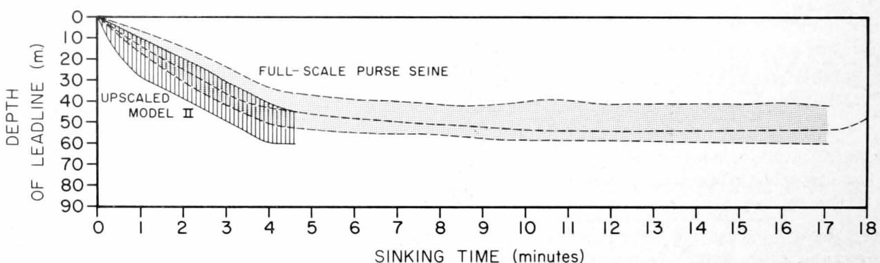
Figure 16.—Predicted sinking performance of scaled up Model II.
