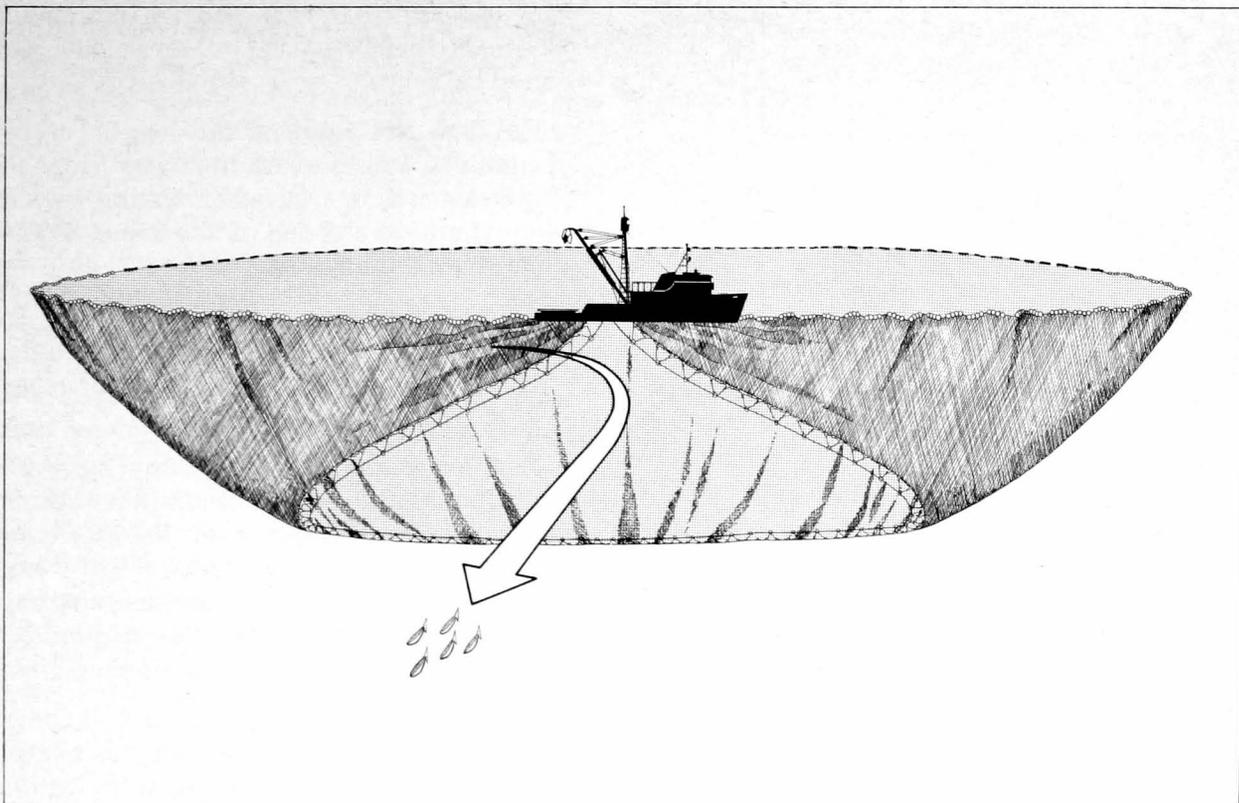
Figure 14.—Fish escape because of unfavorable configuration of partially pursed net.
