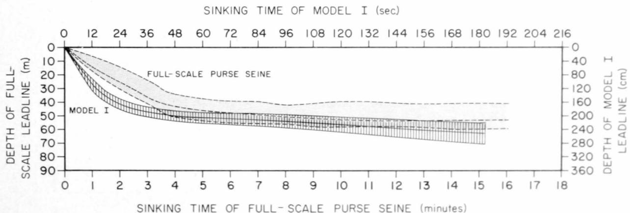
Figure 3.—Comparison of sinking performances at center net of full-scale purse seine and Model I.
