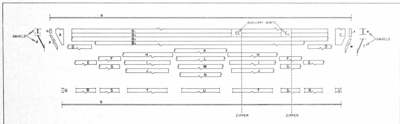
Figure 15.—Construction diagram of hybrid purse seine.
