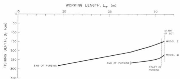
Figure 9.—Relation between working length ( $L_w$ ) and working depth ( $D_w$ ) of each model.
