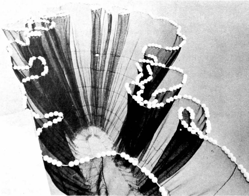
Figure 11.—“Cuplike” configuration in final stage of pursing Model II.
