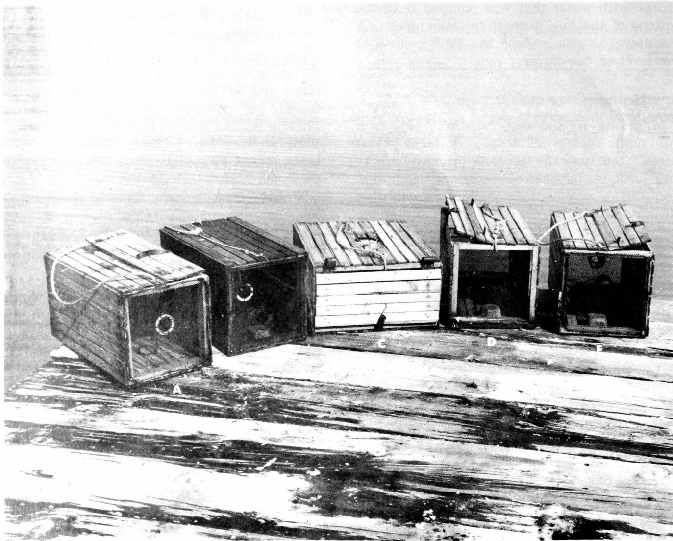
Figure 1.—Shrimp pots with five types of entrances used in efficiency tests: A. Short tunnel; B. Long tunnel; C. Top loader; D. Ramp; E. Plastic pipe.
