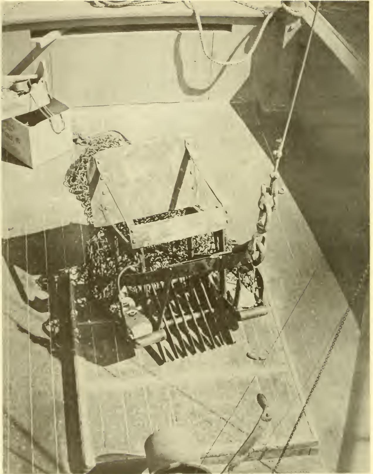
Fig. 3. Hard-shell clam dredges are operated from 30 - 45 foot power boats in the southern half of the Sakonnet River.
