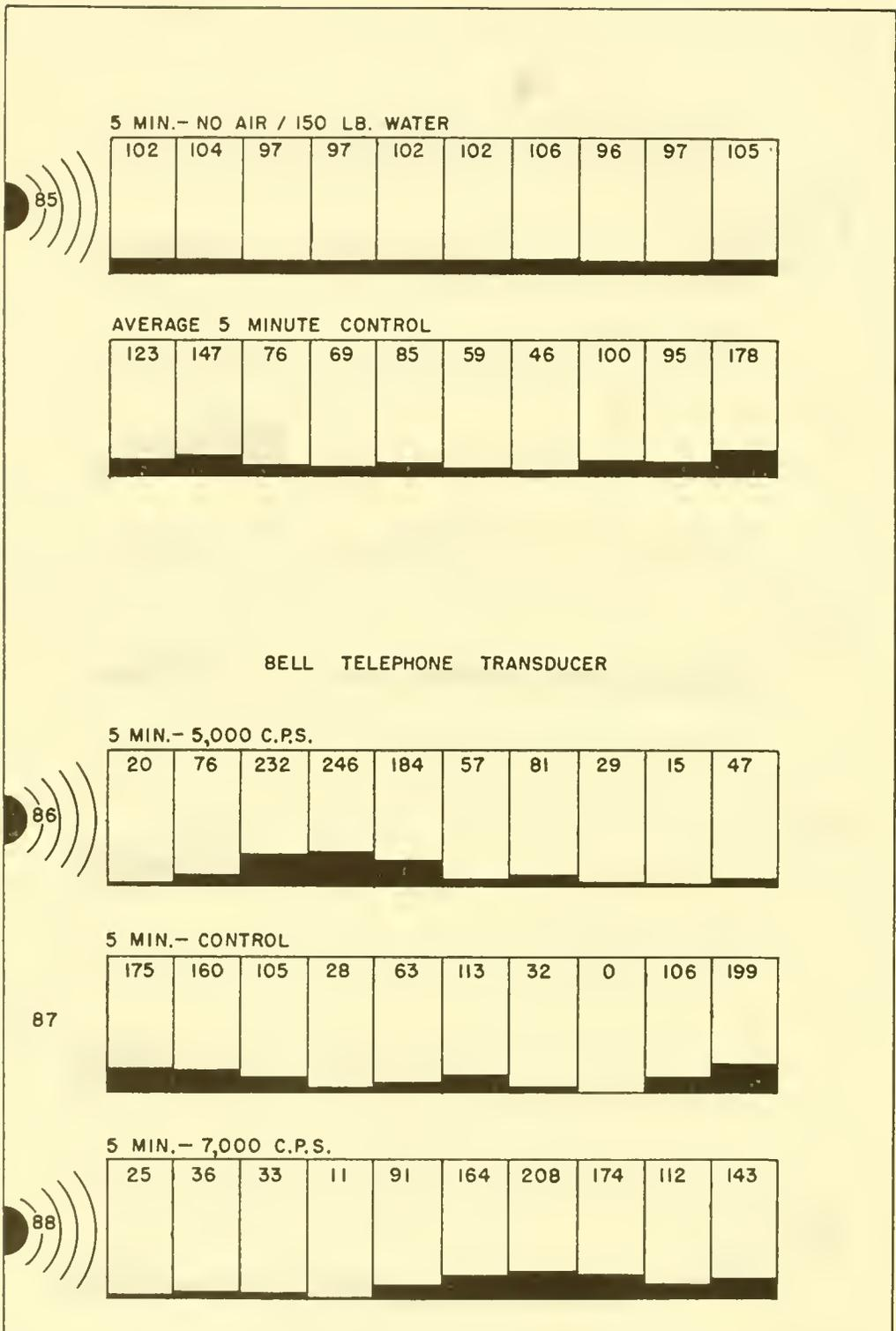
Figure 26. Distribution of fish in pens, experiments 85-88. All experiments started with 100 fish in each pen. In controls, gates between pens lifted for indicated period, then lowered. Tests same, except sounds under indicated operating conditions or at indicated frequencies (cycles per second) applied for indicated time at indicated location. Numbers and dark bars show distribution of fish after gates lowered.
