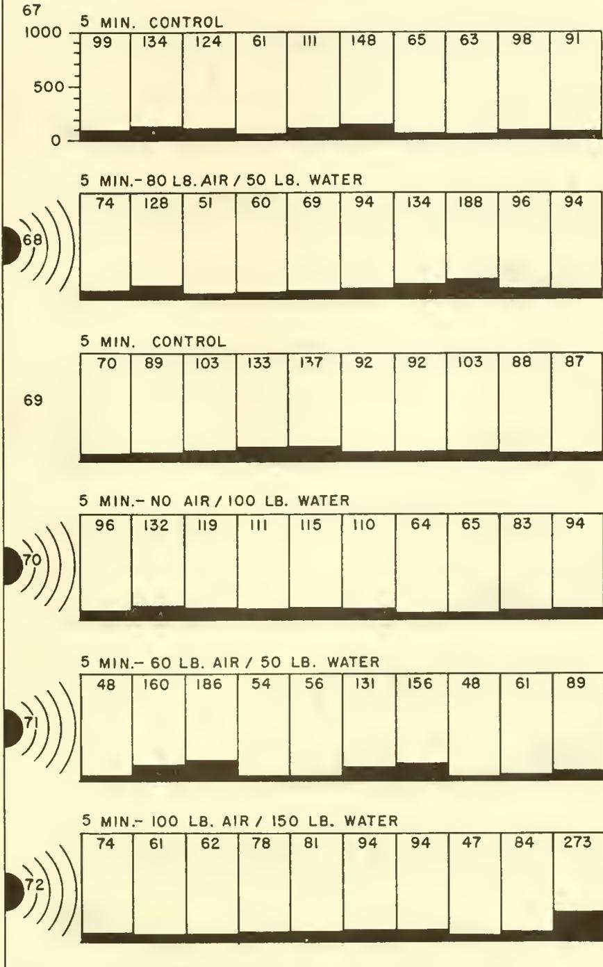
Figure 23. Distribution of fish in pens, experiments 67-72. All experiments started with 100 fish in each pen. In controls, gates between pens lifted for indicated period, then lowered. Tests same, except sounds under indicated operating conditions applied for indicated time at indicated location. Numbers and dark bars show distribution of fish after gates lowered.
