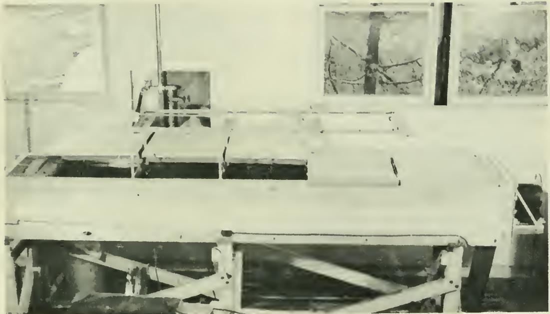
Figure 3. --Experimental tank showing the compartment separators in the "down" position. Note the covers on the tank and the transducer mounted on the end plate. This mounting proved unsatisfactory, and the transducer was later mounted on a separate table.
