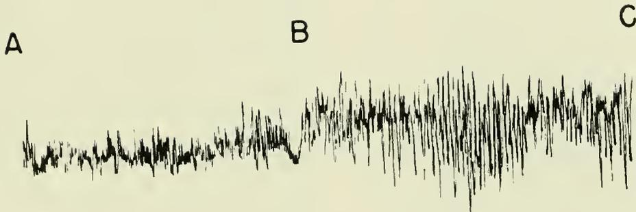
Figure 8. --A tracing of a typical recording of underwater sounds, as received by hydrophone and recorded by wire recorder, then transcribed on the recording voltmeter. The section between "A" and "B" is a recording of ambient noise only; "B" to "C" is a frequency of 20 c.p.s. superimposed upon the ambient noise.
