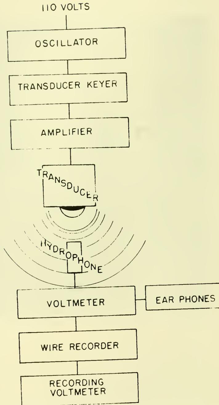
Figure 7. --Block diagram showing electron-unit arrangement.
