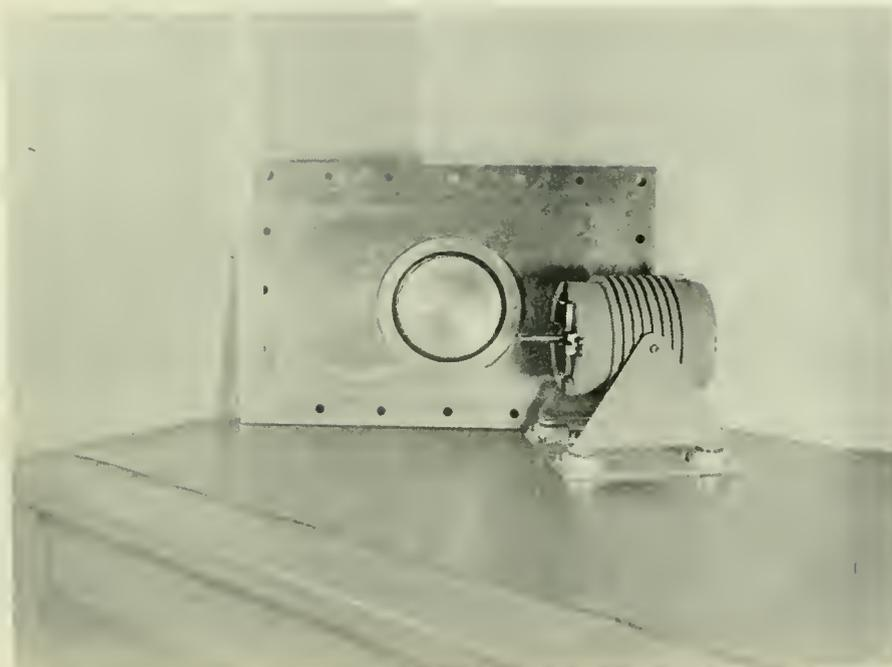
Figure 1. --Electricmagnetic transducer and the end plate from the experimental tank. Note the piston face and the surrounding rubber diaphragm. The piston, when driven by the transducer, created the sound or pressure waves and transferred them into the water. This unit is rated at 100 watts.
