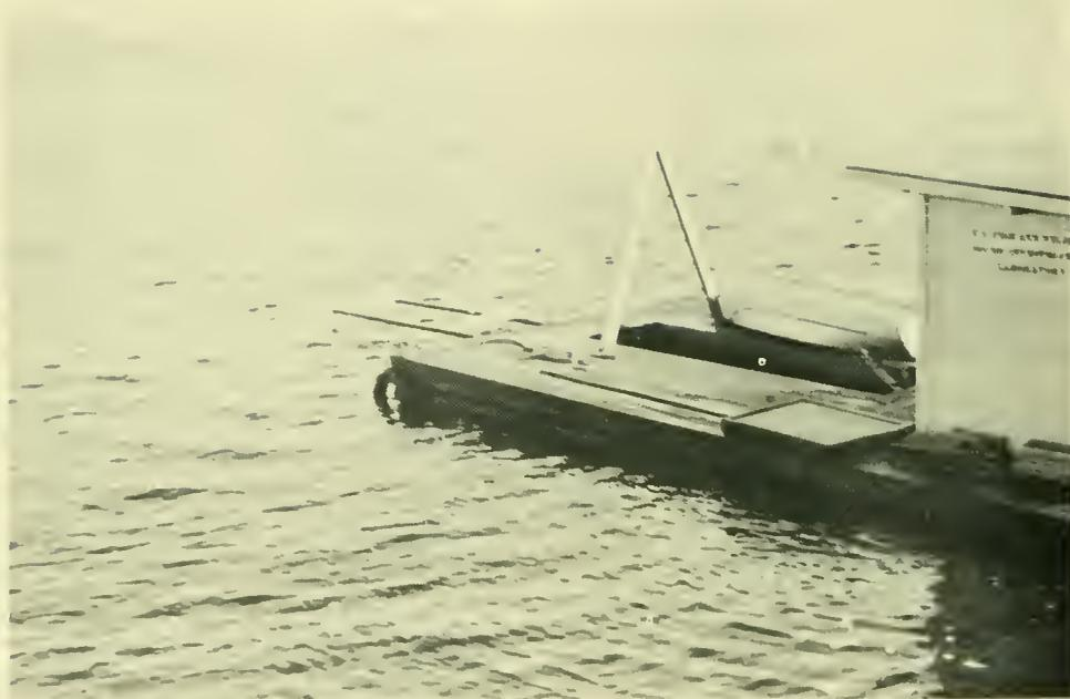
Figure 5.--The floating laboratory on Lake Washington. (Note the rails extending forward, upon which the underwater pen is supported.) The well forward of the cabin allows for easy handling of fish in the pen.
