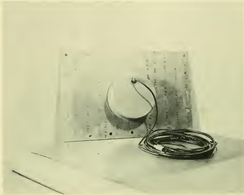
Figure 2. --Piezoelectric transducer mounted in the end plate of the experimental tank. The expansion and contraction of the crystal elements, when energized, creates the sound or pressure waves. These waves are transferred into the water through the front of the "can" which is of thin flexible metal. The "can" is filled with castor oil for more efficient expansion and contraction.
