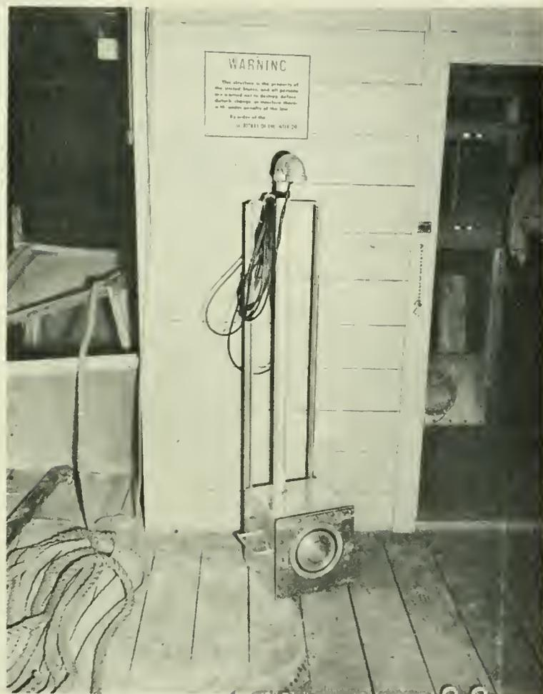
Figure 6. --Watertight aluminum container for submerging the electromagnetic transducer.
