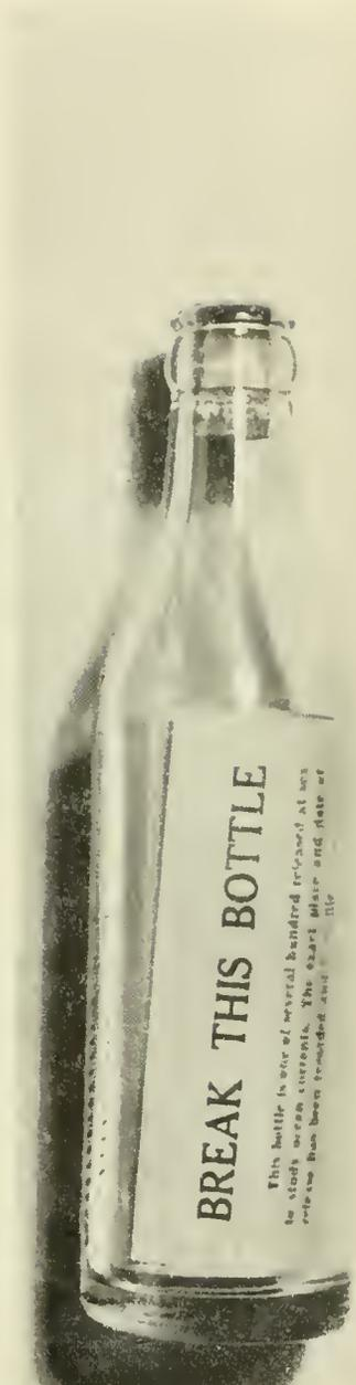
Instead of drogues, dry sand ballast was added to all odd-numbered bottles. Those with even numbers contained no ballast. Six of each were launched at each release station. It was intended that the ballasted bottles float vertically at or near the surface and thus be less influenced by the action of winds and breaking waves. The results, however, indicate no significant difference between the conjectured movement of the two types.
