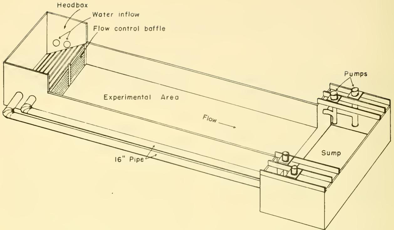
Figure 2.--Main tank showing relation of sump, 40 cfs pumping system and headbox to the experimental area.
