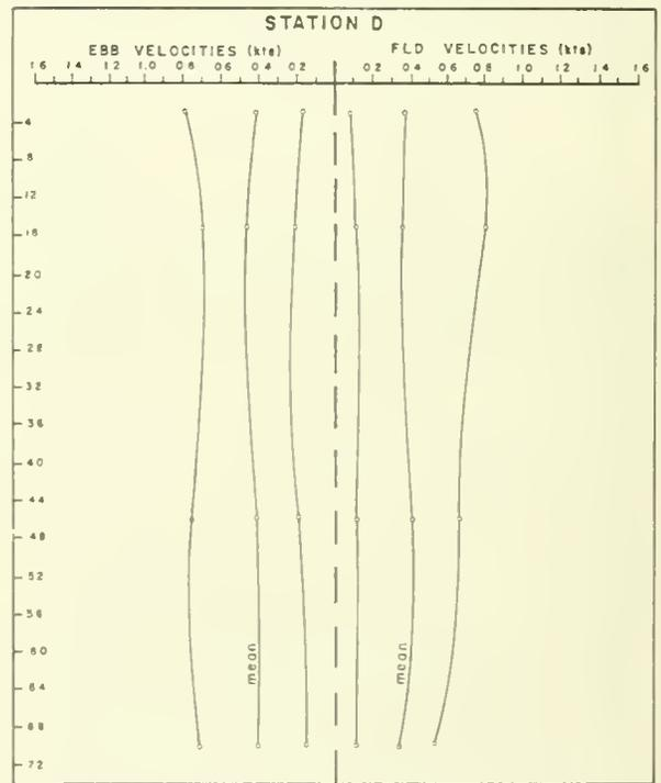
Figure 9.--Mean velocity of the flood and ebb tidal currents observed at each depth on station D. The lines on either side of the means indicate the observed maximum and minimum tidal velocities.
