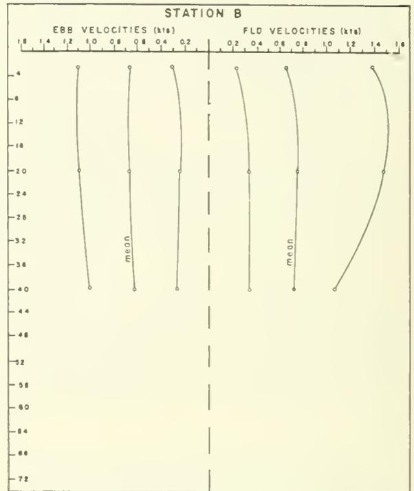
Figure 7.--Mean velocity of the flood and ebb tidal currents observed at each depth on station B. The lines on either side of the means indicate the observed maximum and minimum tidal velocities.
