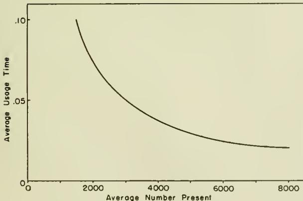
Figure 4.--Relationship between exit rate and number present in a fishway section during a period of constant entry rate.
