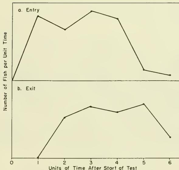
Figure 2.--Distribution in time of fish entering and leaving a test fishway.
