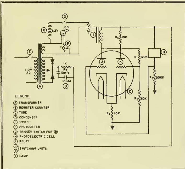
Figure 3.--Electrical diagram of the laboratory current meter.
