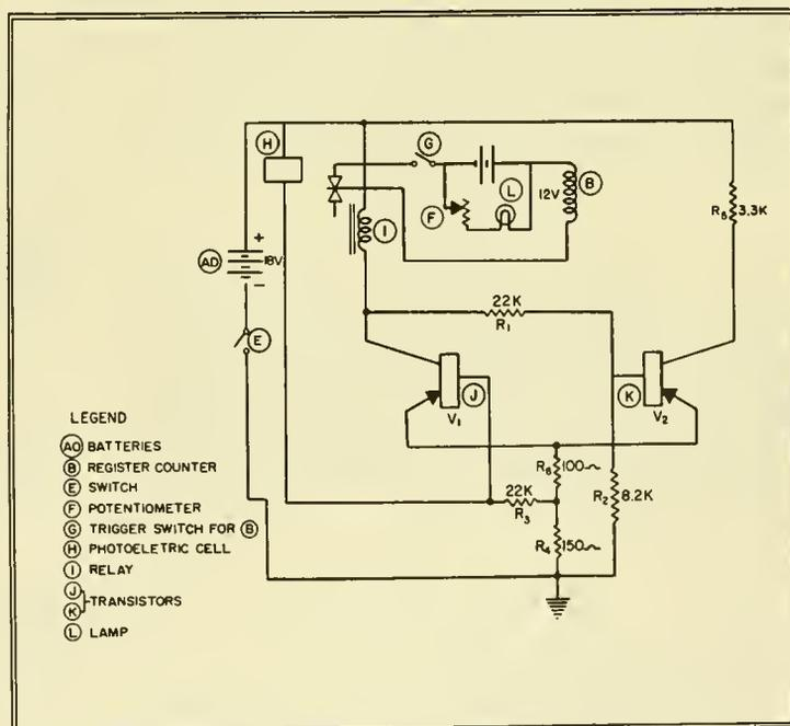
Figure 5.--Electrical diagram of the field current meter.
